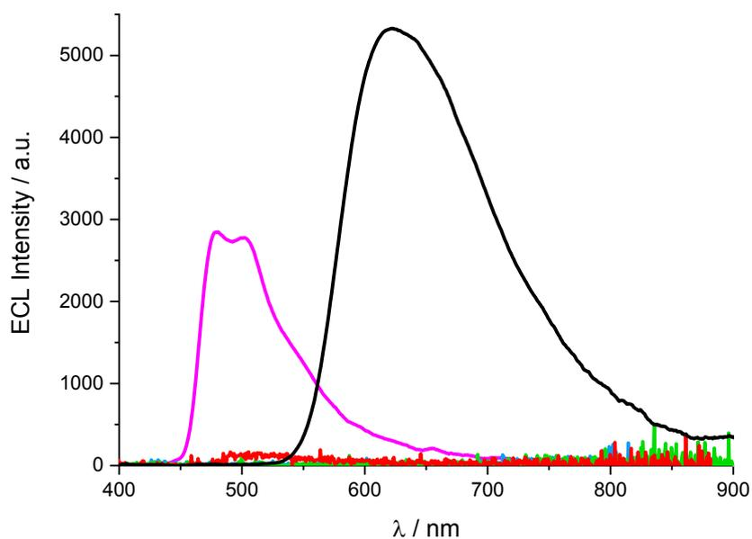
**Figure S2.** Co-reactant ECL spectra for the complexes **7-9** and **11** (1 mM) in acetonitrile containing 0.1 M  $[\text{Bu}_4\text{N}][\text{PF}_6]$  as supporting electrolyte and 10 mM tripropylamine (TPA) as the co-reactant. (green) **7**; (pink) **8**; (blue) **9**; (red) **11**; (black)  $[\text{Ru}(\text{bpy})_3]^{2+}$ .
