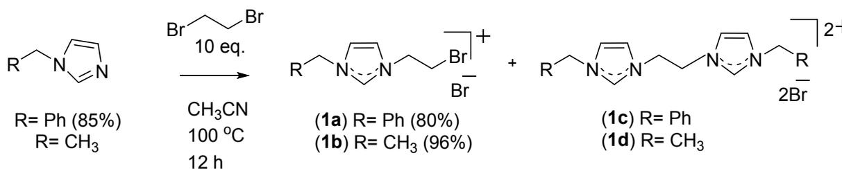
**Scheme S1.** Synthesis of imidazolium salts **1a** and **1b** (with their corresponding bis-imidazolium salt biproducts **1c** and **1d**, respectively).
