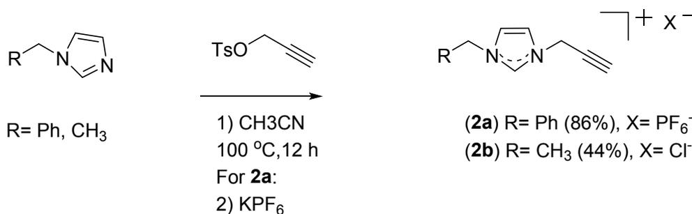
**Scheme S2.** Synthesis of the alkyne functionalized imidazolium salts **2a** and **2b**.
