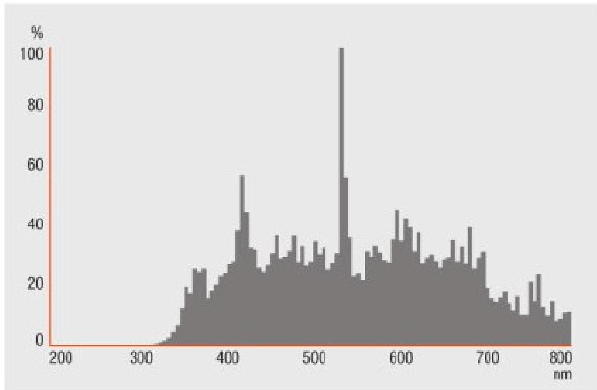
**Figure S79.** Optical emission spectrum of the 400 W Powerstat HQI BT MM (Osram) tungsten lamp used for the photobleaching studies (picture provided by the courtesy of the manufacturer).
