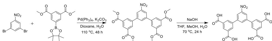
**Scheme S1** Synthetic procedure of H<sub>4</sub>DDPN.
