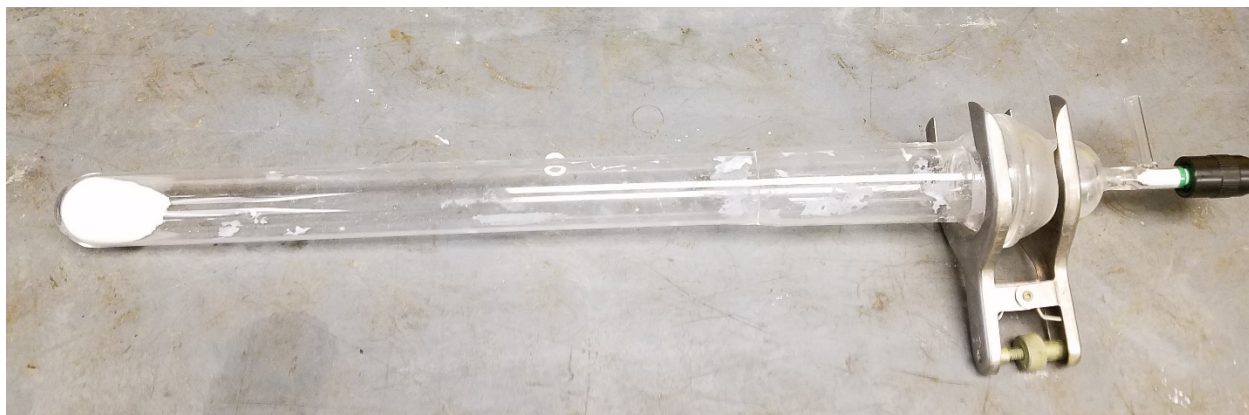
Figure S1. Quartz tube utilized for tube furnace preparation of \text{SiO}_2^{700} , including heating to 700 °C under vacuum.
