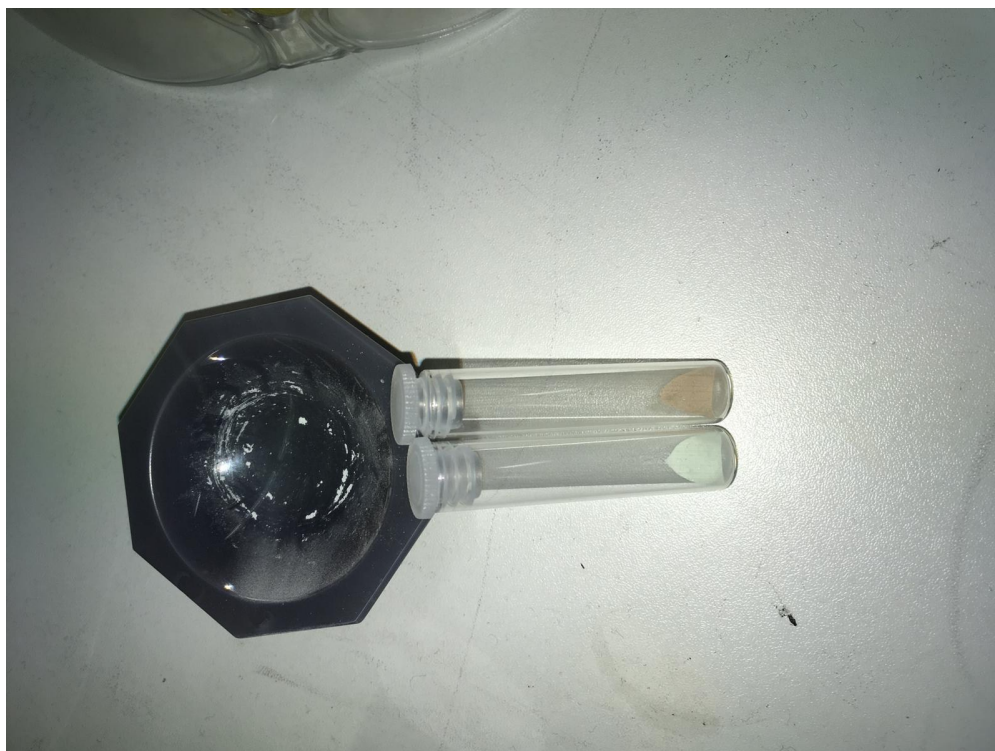
Fig. S7 Colour change of activated CFA-15 after treatment with NO.
