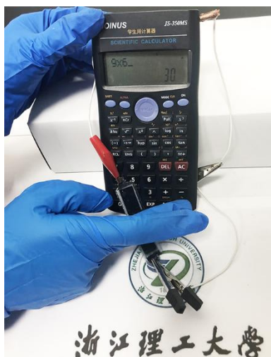
Figure S6. The photograph of two assembled flexible solid-state HSC devices connected in series as the power for the calculator.
