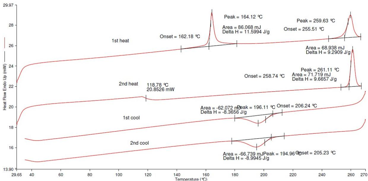
Figure S4. DSC of  $\text{SO}_2@Cr_8$
