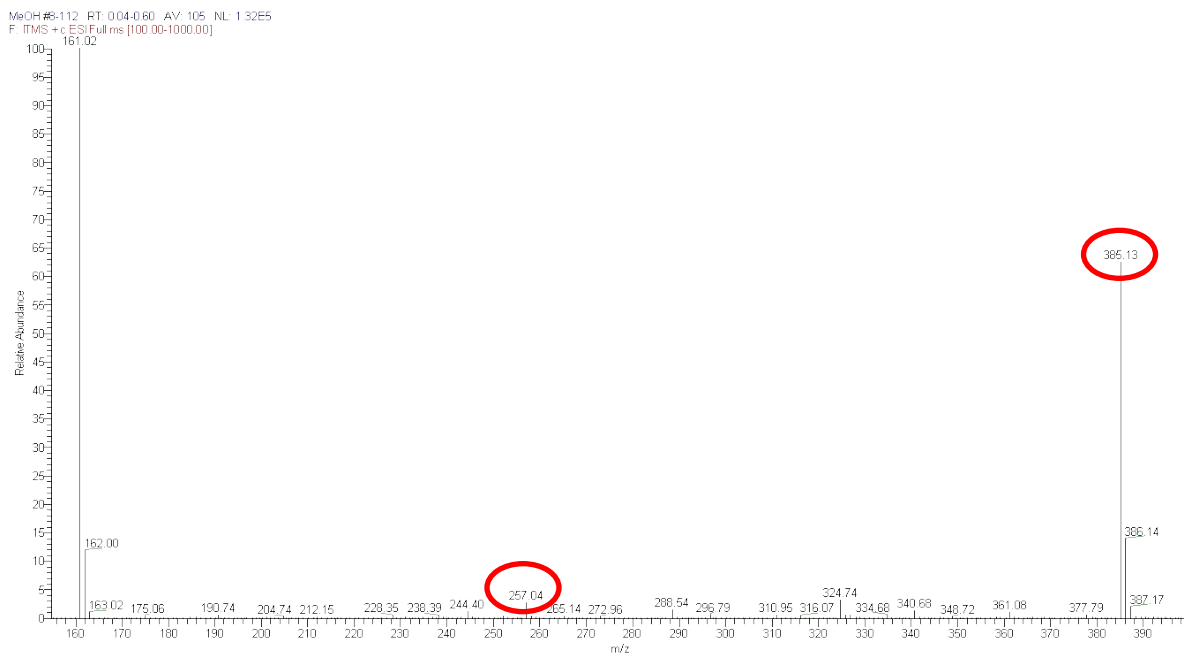
Fig. S13C. ESI-MS(+) [ V^{IV}O(PIMH)_2 ] in methanol after 48 h dissolution (peak at m/z = 385.13 ).
