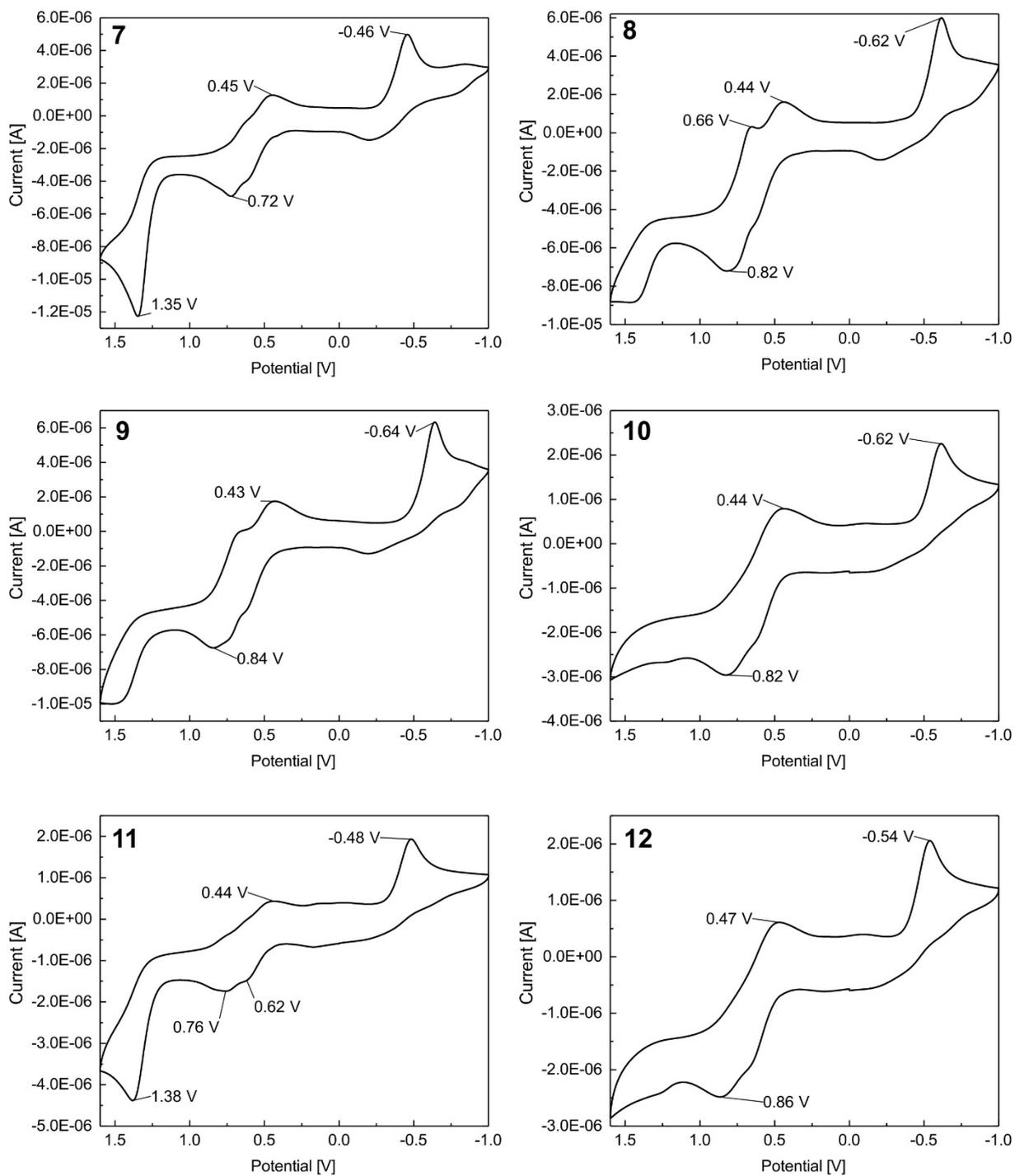
**Figure S12.** Cyclic voltammograms (MeCN, 0.1 M  $\text{NBu}_4\text{PF}_6$ , vs.  $\text{Ag}/\text{AgNO}_3$ , 50 mV/s) of **13–18**.
