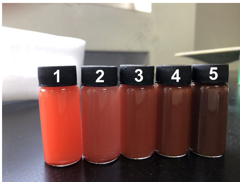
Figure. S5 The photographs of (1) Ta 3 N 5 , (2) Ta 3 N 5 /MoS 2 -1, (3) Ta 3 N 5 /MoS 2 -2, (4) Ta 3 N 5 /MoS 2 -3 and (5) Ta 3 N 5 /MoS 2 -4 aqueous solution.
