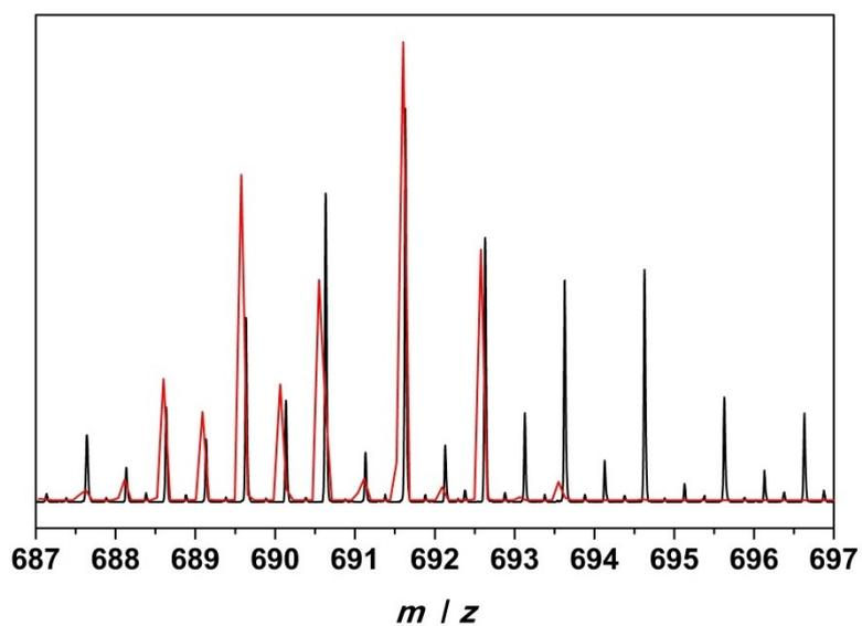
**Fig. S10** Simulated (red) and experimental (black) negative-mode mass spectra of isotopic envelopes for compound **1**.
