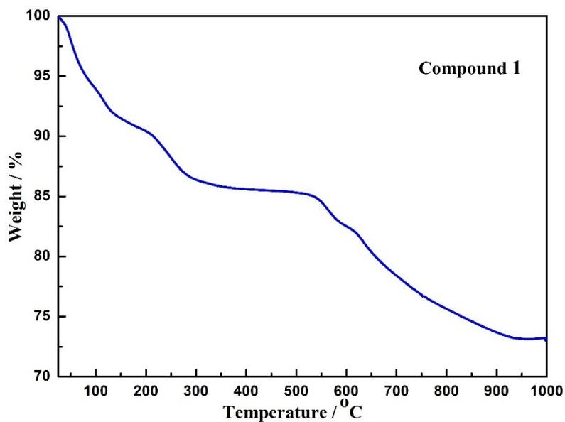
**Fig. S8** The TG curves of **1** were measured in the range of 25-1000 °C under nitrogen gas atmosphere with the heating rate of 10 °C/min.
