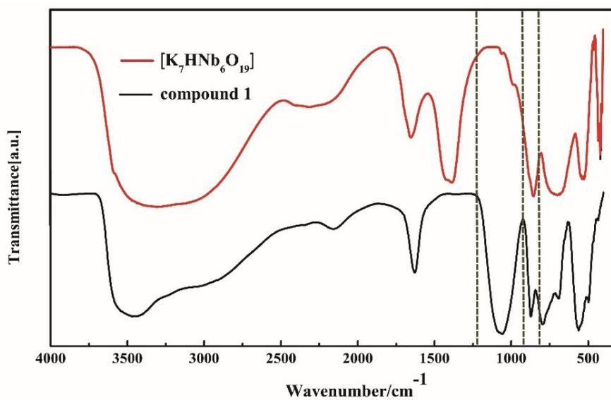
**Fig. S7** IR spectra of  $K_7HNB_6O_{19} \cdot 13H_2O$  and compound **1**.
