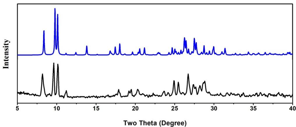
**Fig. S6** The PXRD pattern (bottom) of **1** and its calculated pattern (top) based on the single-crystal solution.
