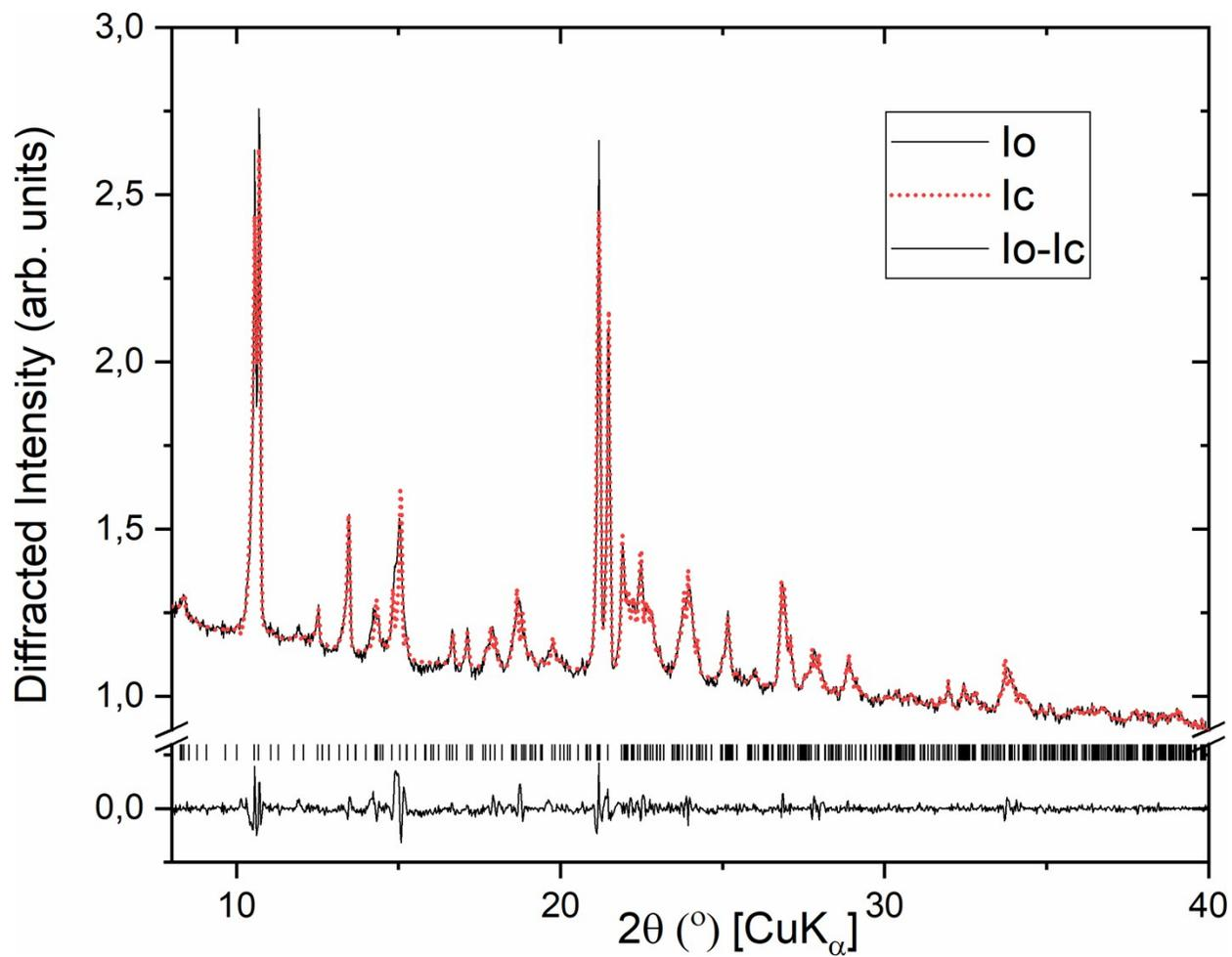
Figure S2. The results of the Le Bail refinement of the unit cell and profile parameters for TriBuMeFe. The red line stands for the calculated intensity; the difference plot is drawn in the bottom. Black sticks show positions of the Bragg peaks;  $a=19.537(2)\text{\AA}$ ,  $b=13.165(2)\text{\AA}$ ,  $c=20.233(2)\text{\AA}$ ,  $\beta=115.3(1)^\circ$ ,  $V=4705(1)\text{\AA}^3$ ;  $R_p=1.35$ ,  $wR_p= 2.08$ .
