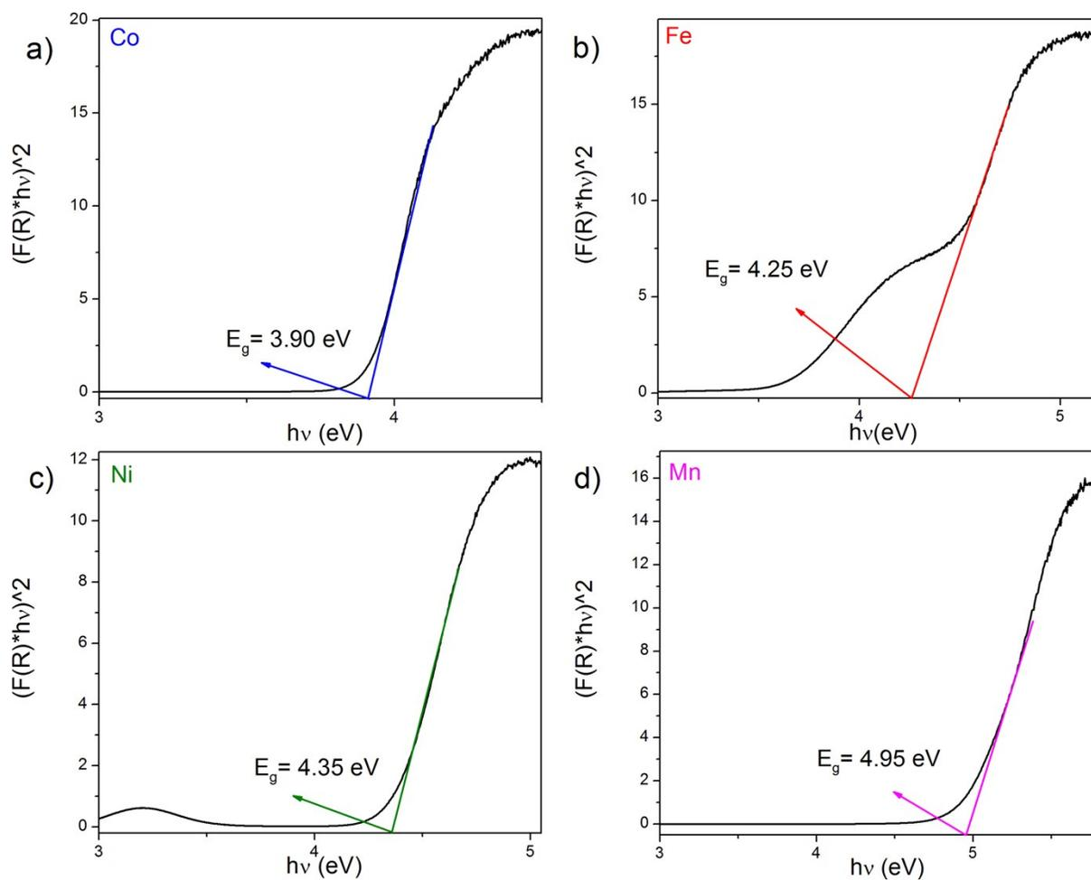
Figure S17. The energy band gap of TriBuMeM, (M= Fe, Co, Ni, Mn) determined using Kubelka – Munk function.
