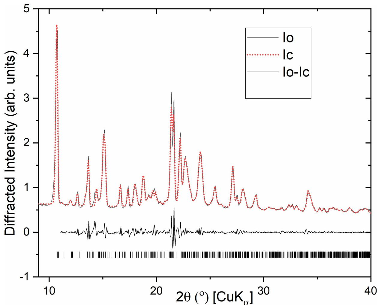
Figure S4. The results of the Le Bail refinement for TBuMeANi\_dca. The red line stands for the calculated intensity; the difference plot is drawn in the bottom. Black sticks show positions of the Bragg peaks;  $a=19.41(2)\text{\AA}$ ,  $b=12.81(2)\text{\AA}$ ,  $c=19.64(2)\text{\AA}$ ,  $\beta=114.7(1)^\circ$ ,  $V=4737(30)\text{\AA}^3$ ;  $R_p=3.63$ ,  $wR_p=6.45$ .  $I_o$  of the most intense peak is disrupted by the texture, thus the  $I_o - I_c$  is not presented for the picture clarity.
