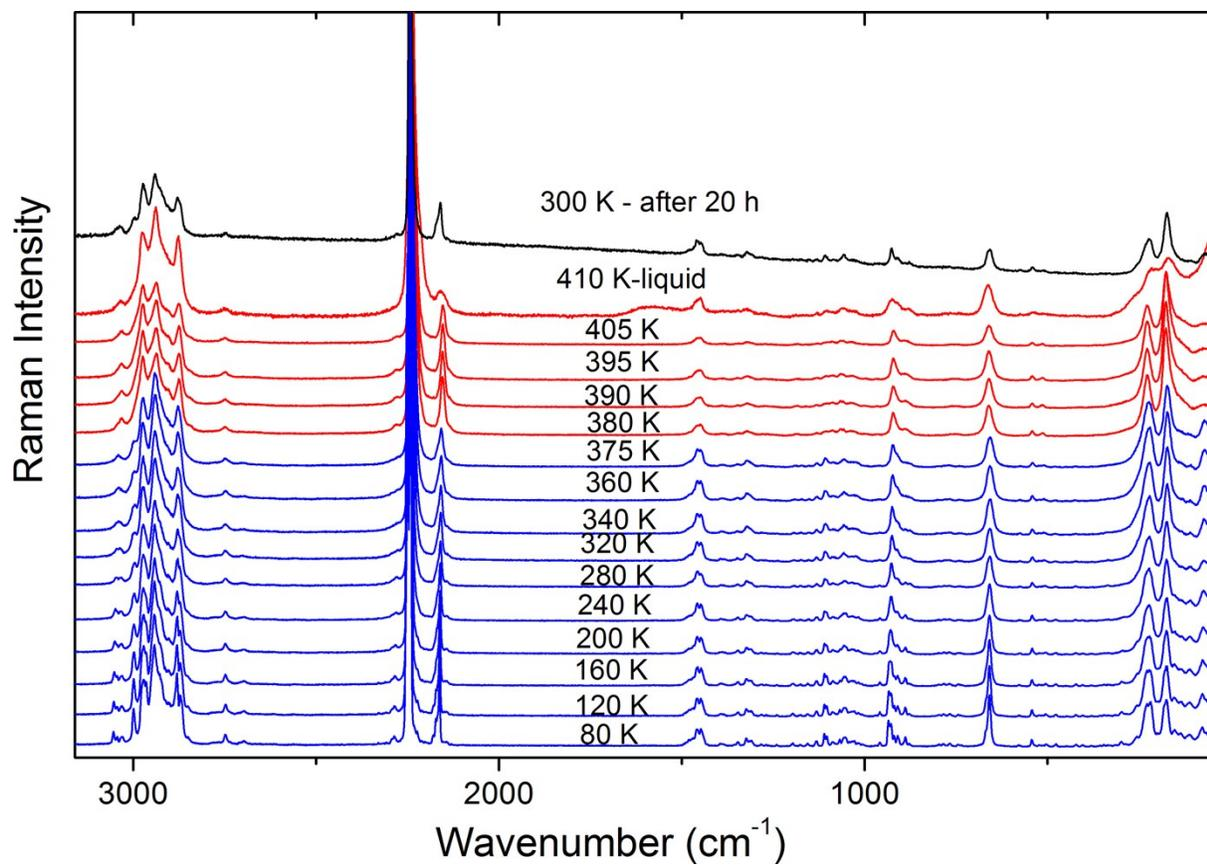
Figure S13. Temperature-dependent Raman spectra of TriBuMn in the whole wavenumber range.
