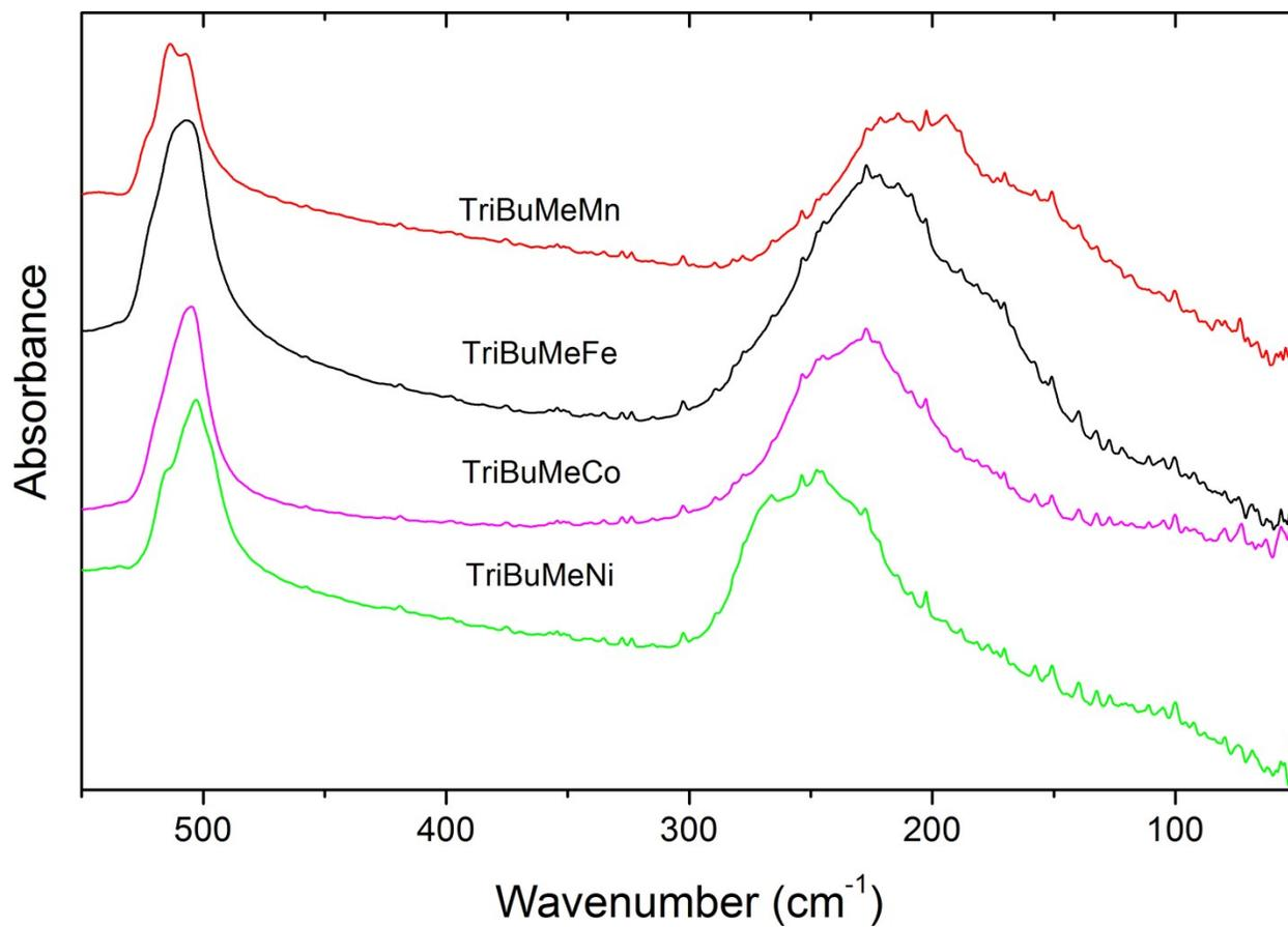
Figure S12. Far-IR spectra of TriBuMeM samples at room temperature.
