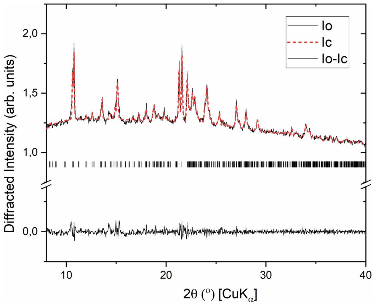
Figure S3. The results of the Le Bail refinement for TriBuMeCo. The red line stands for the calculated intensity; the difference plot is drawn in the bottom. Black sticks show positions of the Bragg peaks;  $a=19.706(2)\text{\AA}$ ,  $b=13.029(2)\text{\AA}$ ,  $c=19.845(2)\text{\AA}$ ,  $\beta=115.0(1)^\circ$ ,  $V=4617.8(6)\text{\AA}^3$ ;  $R_p=1.05$ ,  $wR_p= 1.55$ .
