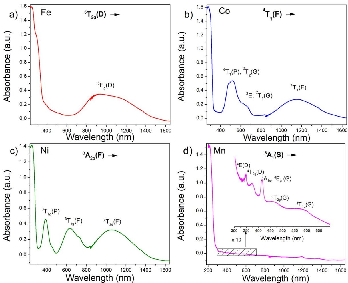
Figure S16. Absorption spectra of a) TriBuMeFe b) TriBuMeCo c) TriBuMeNi and d) TriBuMeMn recorded at 300 K.
