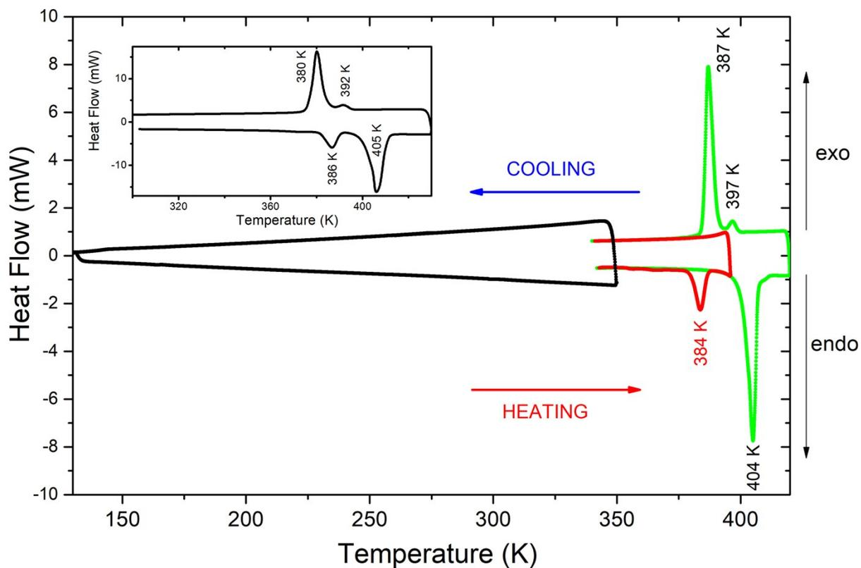
Figure S5. DSC traces for TriBuMeMn: heating up to 396 K and cooling to 340 K (1<sup>st</sup> run, red line) followed by heating to 420 K and cooling to 340 K (green, 2<sup>nd</sup> run). Inset shows DSC trace of new sample heated to 430 K and cooled down to RT.
