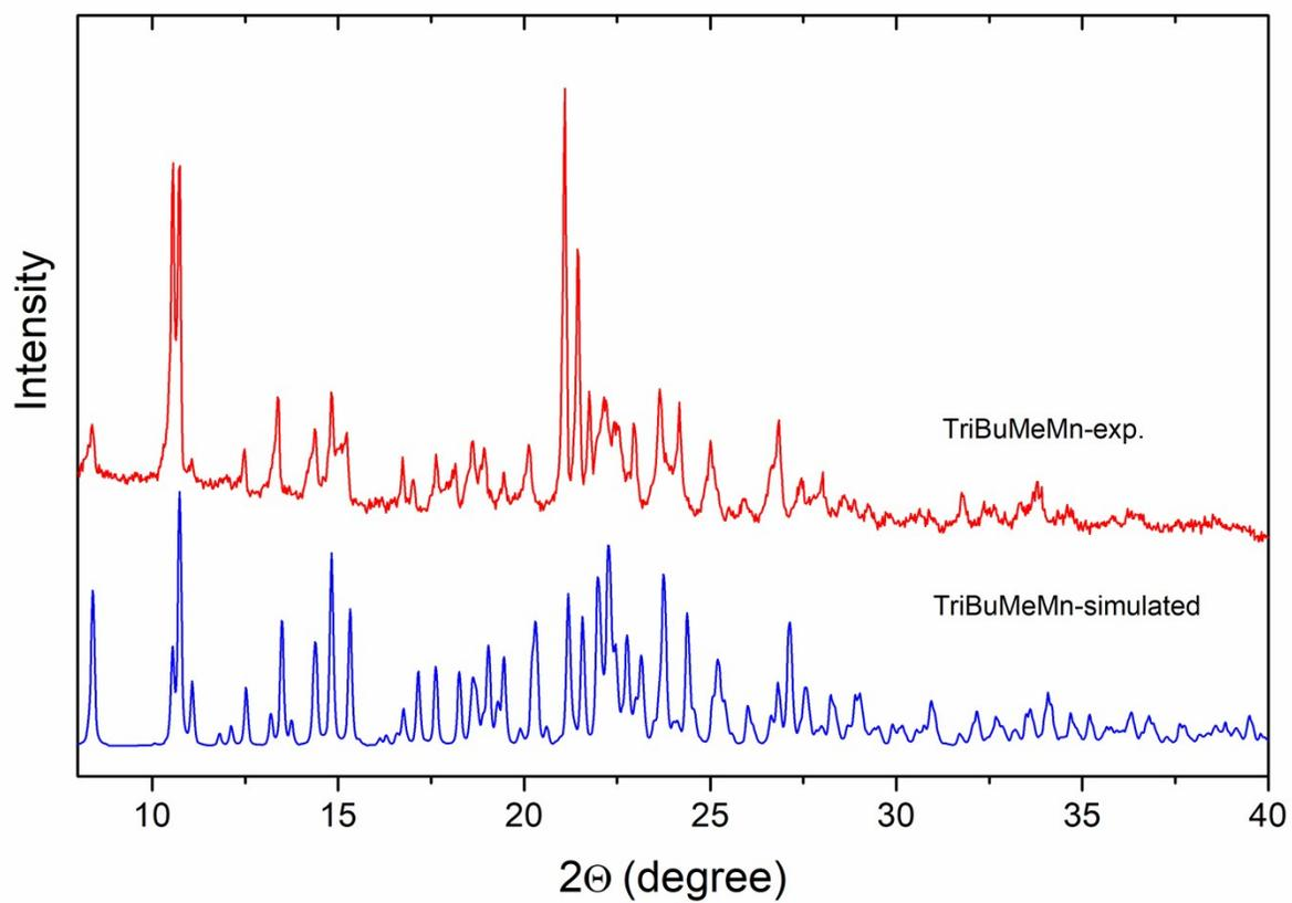
Figure S1. Room-temperature powder XRD pattern for the as-prepared TriBuMeMn sample together with the calculated one based on the single crystal structure.
