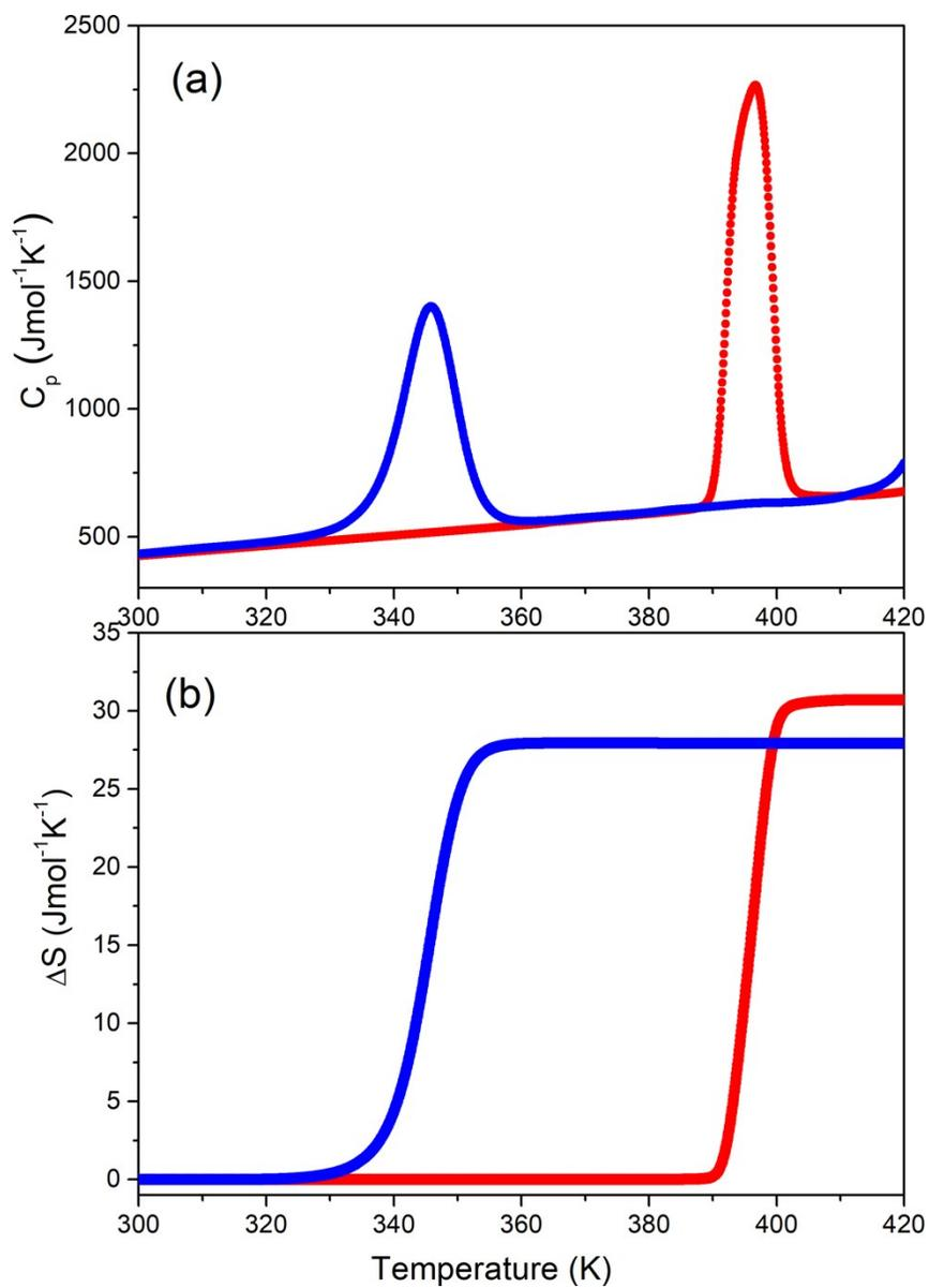
Figure S7. Temperature dependence of (a)  $C_p$  and (b)  $\Delta S$  related to the phase transitions in TriBuMeNi in heating (red) and cooling (blue) run.
