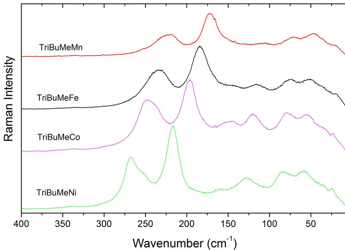
Figure S10. Raman spectra of TriBuMeM samples measured with use of eclipse filter to show low-wavenumber region down to  $5 \text{ cm}^{-1}$ .
