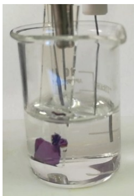
Fig. S9. Three electrodes system of electrochromic measurement.
