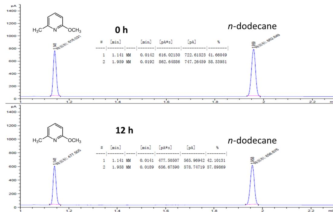
Fig. S43 GC analysis for Reaction of  $\text{RuHCl}(\text{PPh}_3)_3(\text{CO})$  with 2-methoxy-6-methylpyridine.
