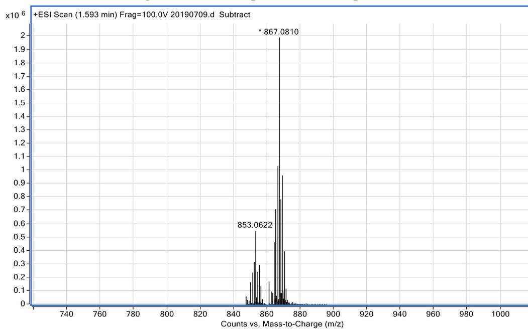
Fig. S39 Reaction of complex **1** with H<sub>2</sub><sup>18</sup>O (The peak at 853.0622 ([M+H]<sup>+</sup>) belongs to **2**, and the peak at 867.0810 ([M-Cl]<sup>+</sup>) belongs to the cation of **1**).
