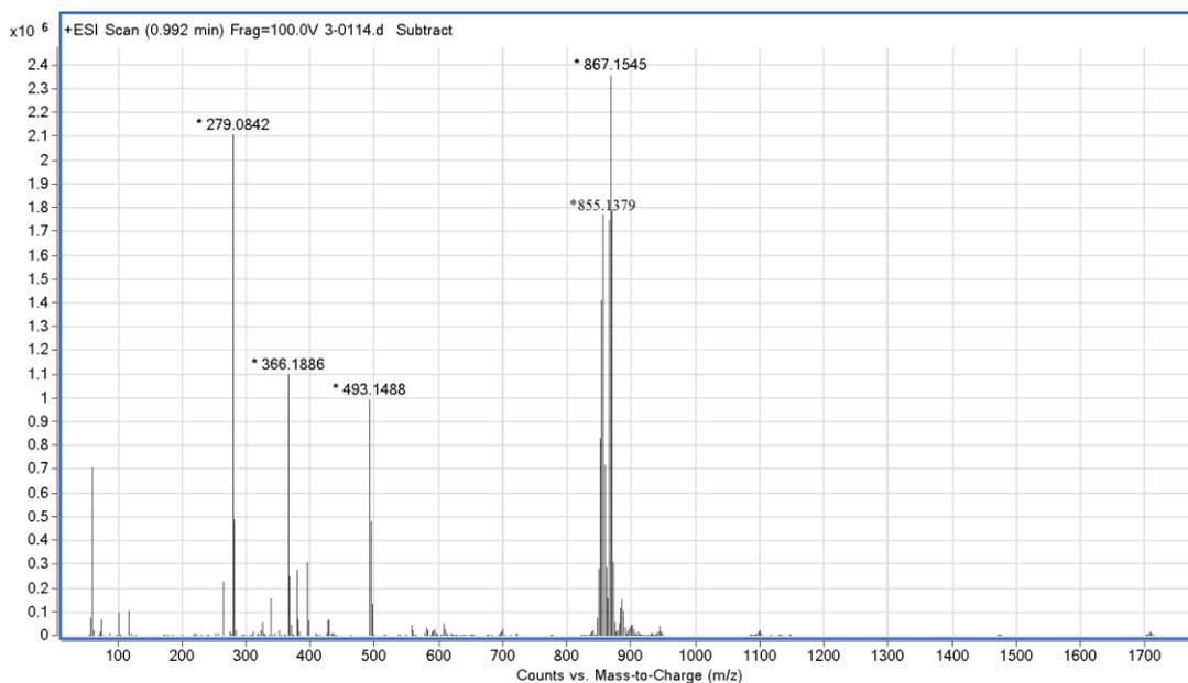
Fig. S40 Reaction of complex **1** with KOH/H<sub>2</sub><sup>18</sup>O (The peak at 855.1379 ([M+H]<sup>+</sup>) belongs to the <sup>18</sup>O-substituted **2**, and the peak at 867.1545 ([M-Cl]<sup>+</sup>) belongs to the cation of **1**).
