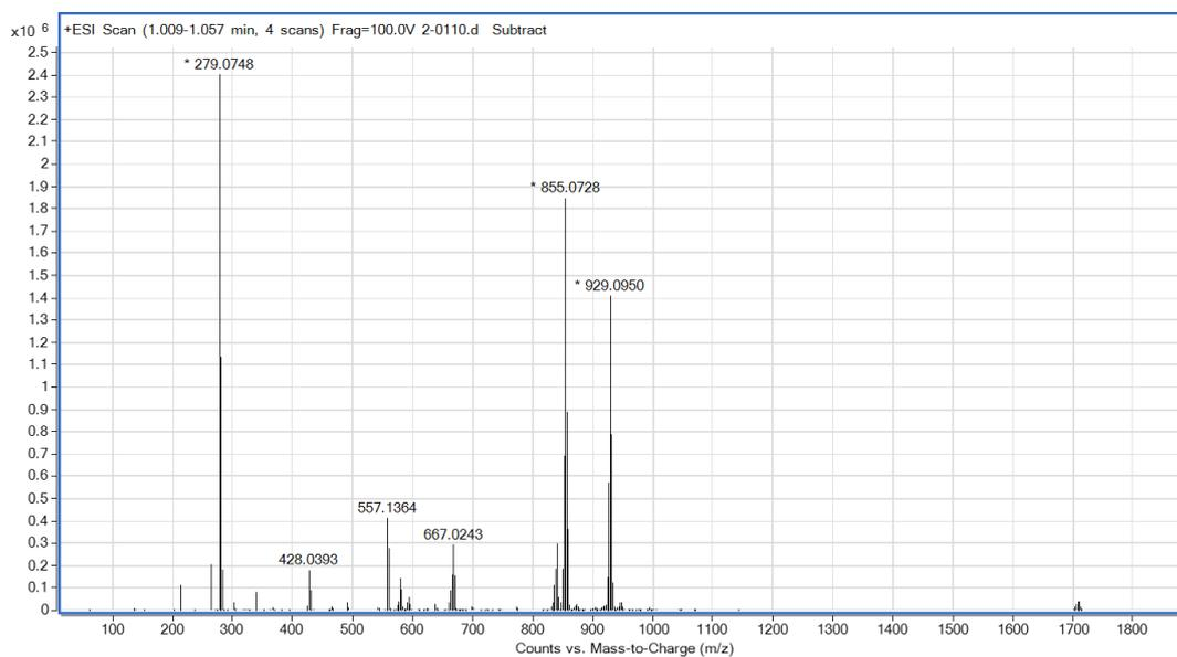
Fig. S41 Reaction of complex **3** with KOH/H<sub>2</sub><sup>18</sup>O (The peak at 855.0728 ([M+H]<sup>+</sup>) belongs to the <sup>18</sup>O-substituted **2**, and the peak at 929.0950 ([M-Cl]<sup>+</sup>) belongs to the cation of **3**).
