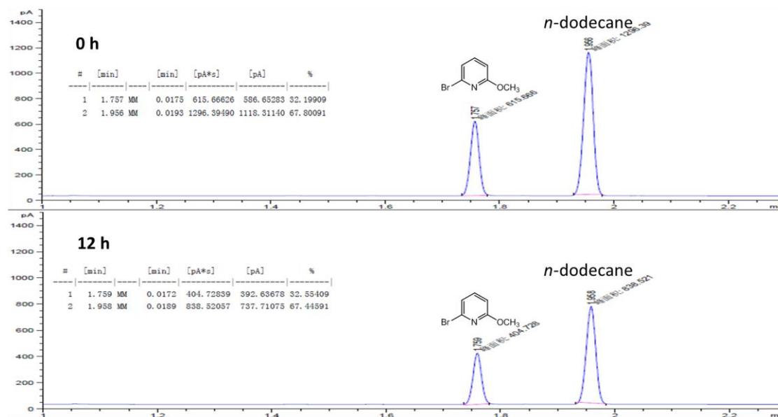
Fig. S42 GC analysis for Reaction of  $\text{RuHCl}(\text{PPh}_3)_3(\text{CO})$  with 2-bromo-6-methoxypyridine.
