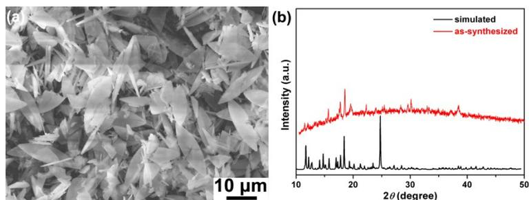
**Fig. S1** (a) SEM images of pure MOF and (b) XRD patterns of Co-MOF.
