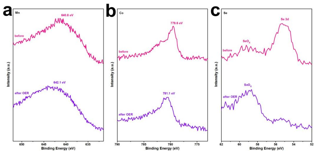
**Fig. S4** High resolution XPS spectra of (a) Mn 2p<sub>3/2</sub>, (b) Co 2p<sub>3/2</sub> and (c) Se 3d of as-prepared and post-OER Mn-CoSe<sub>2</sub>/NF catalysts.
