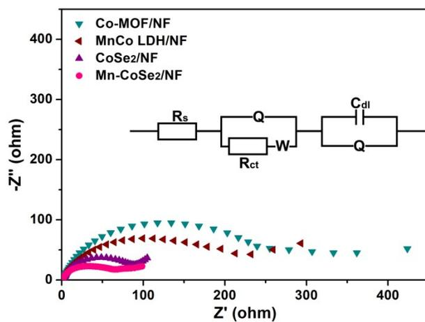
**Fig. S2** Nyquist plots of Co-MOF, MnCo LDH, CoSe<sub>2</sub> and Mn-CoSe<sub>2</sub>/NF catalysts (inset: equivalent circuit model).
