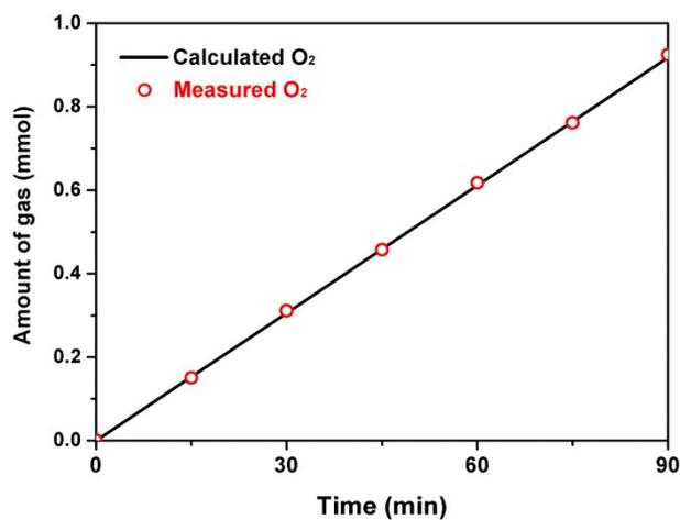
Fig. S7 O<sub>2</sub> production amount of the theoretically calculated and experimentally measured versus time for Mn-CoSe<sub>2</sub> catalysts at 60 mA cm<sup>-2</sup>.
