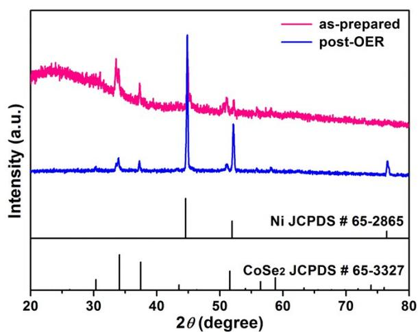
Fig. S6 XRD patterns of as-prepared and post-OER Mn-CoSe<sub>2</sub>/NF catalysts.
