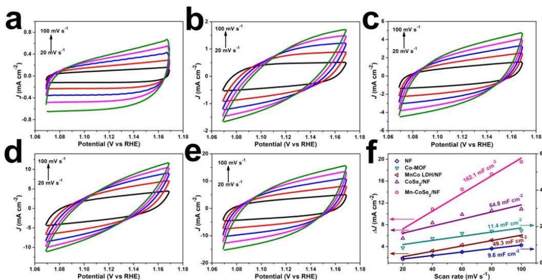
**Fig. S3** Cyclic voltammetry curves at different scan rates for (a) NF, (b) Co-MOF/NF, (c) MnCo LDH/NF, (d) CoSe<sub>2</sub>/NF and (e) Mn-CoSe<sub>2</sub>/NF catalysts. (f) Corresponding linear relationship between current density differences and scan rate.
