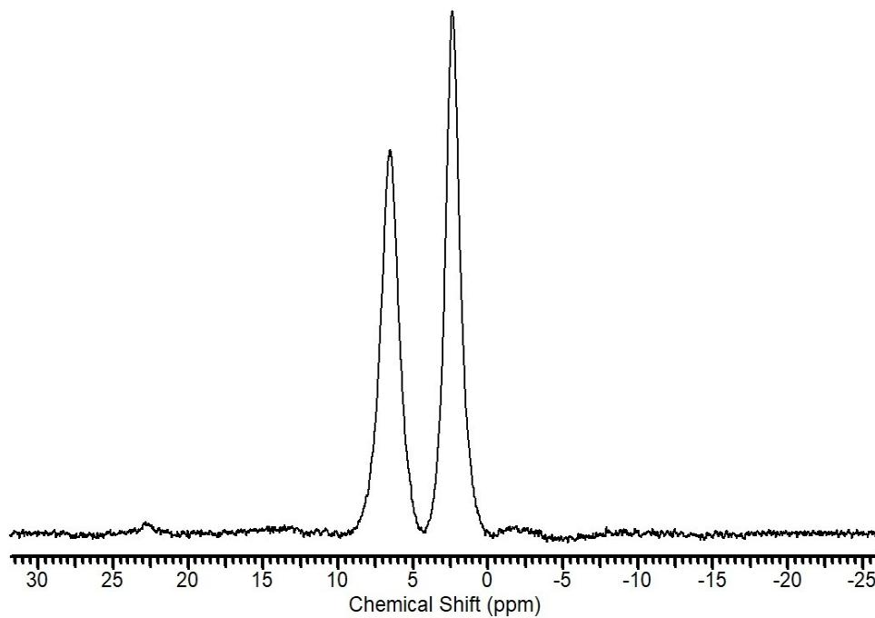
$^{19}\text{F}$  NMR spectrum (376 MHz,  $\text{CD}_2\text{Cl}_2$ ) for **4**(OTf).
