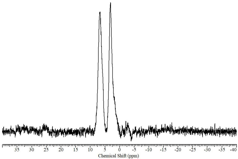
$^{19}\text{F}$  NMR spectrum (376 MHz,  $\text{CD}_2\text{Cl}_2$ ) for **5(OTf)**.
