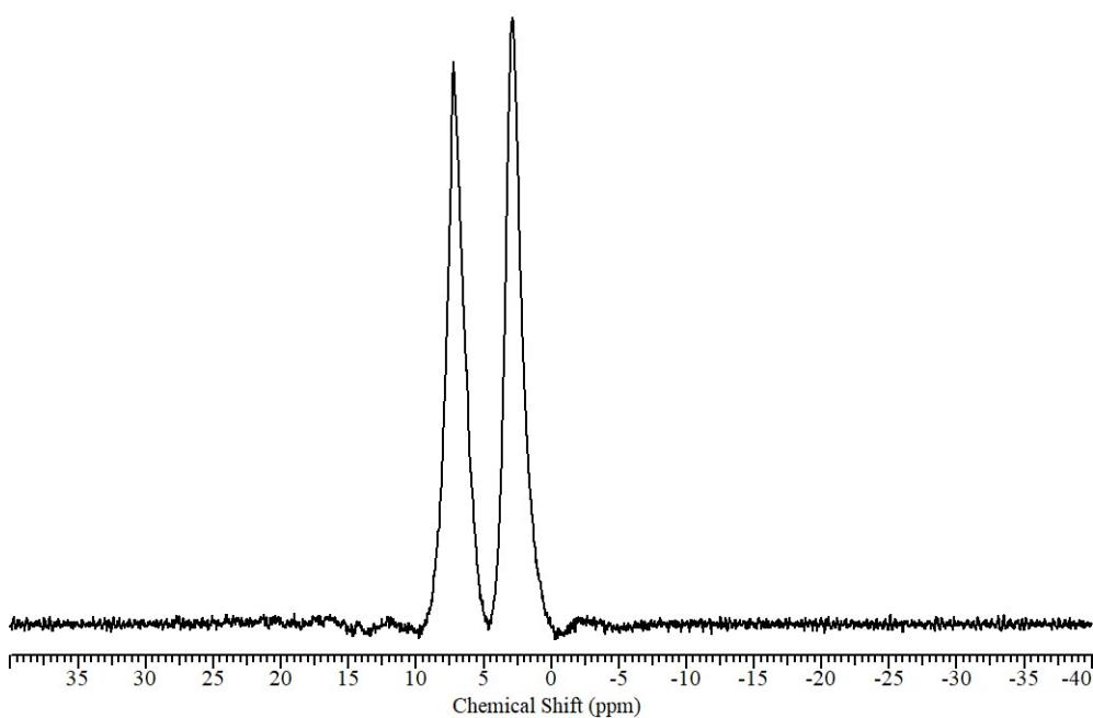
$^{19}\text{F}$  NMR spectrum (376 MHz,  $\text{CD}_2\text{Cl}_2$ ) for **6**(OTf).
