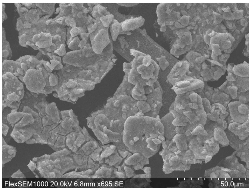
Figure S13. SEM image of larger aggregates of the ternary tetraselenomolybdates, after toluene extraction of samples synthesized from a 4:1 Cu:Mo reaction at a 200 °C injection temperature and isolated after 5 min.
