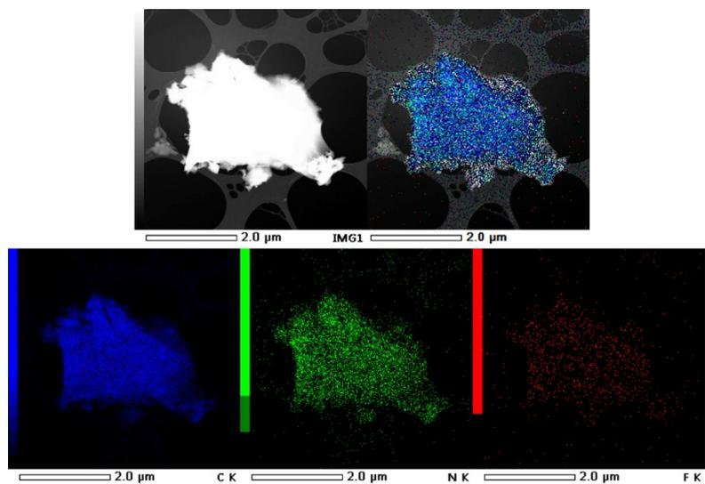
Figure S6. High angle annular dark field scanning-transmission electron microscopy (HAADF-STEM) and corresponding energy dispersive X-ray spectroscopy (EDX) mapping images of carbon (blue), nitrogen (green) and fluorine (red) for the sample FCTF-20-400.
