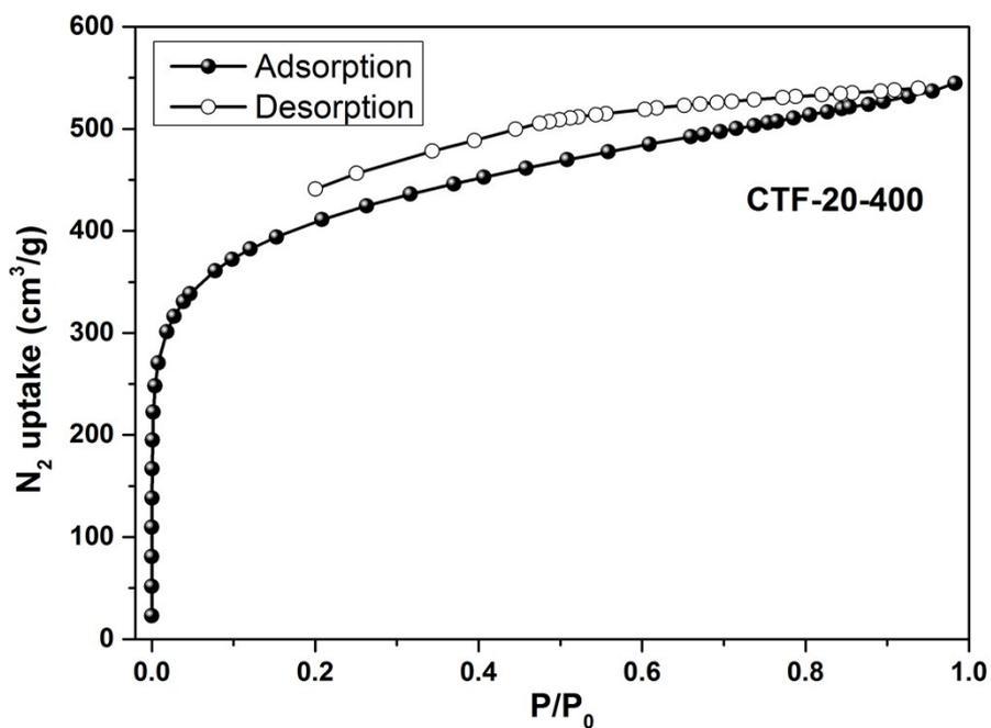
Figure S11. N<sub>2</sub> adsorption (solid symbols) and desorption (empty symbols) isotherm of CTF-20-400.
