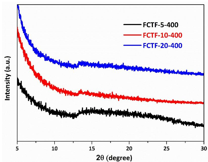
Figure S4. Powder X-ray diffraction (PXRD) patterns of all obtained CTF materials.
