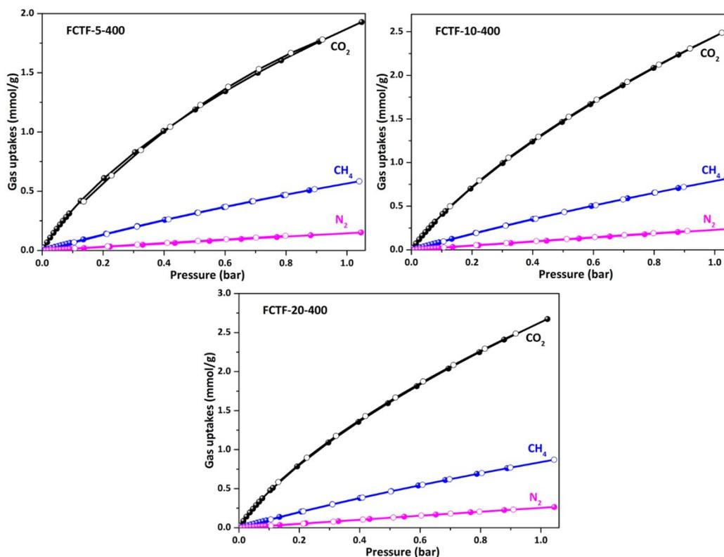
Figure S13. CO<sub>2</sub>, CH<sub>4</sub> and N<sub>2</sub> adsorption isotherms for all the obtained fluorinated CTFs measured at 298 K up to 1 bar.
