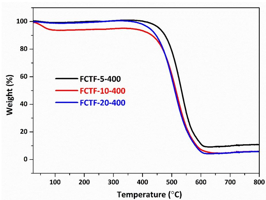
Figure S10. TGA curves of the studied FCTF materials measured at a heating rate of 5 °C/min under an air flow.
