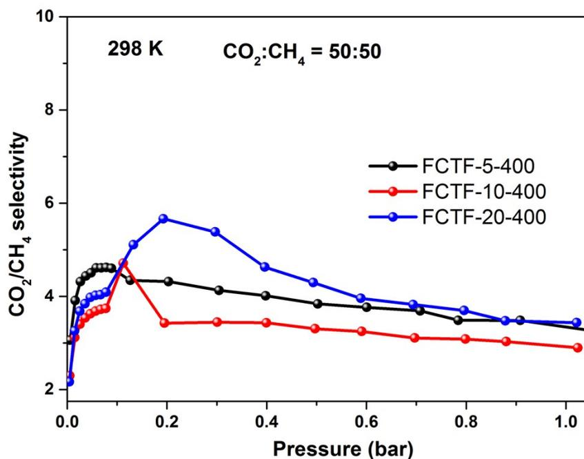
Figure S18: Calculated IAST selectivity of binary gas mixtures ( $\text{CO}_2:\text{CH}_4 = 50:50$ ) at 298 K for all the studied FCTFs.
