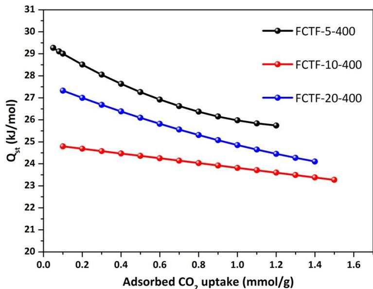
Figure S14. The isosteric heat of CO<sub>2</sub> adsorption ( $Q_{st}$ ) for all FCTF materials.
