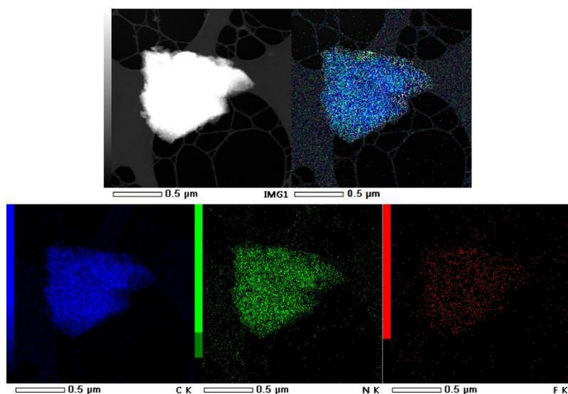
Figure S5. High angle annular dark field scanning-transmission electron microscopy (HAADF-STEM) and corresponding energy dispersive X-ray spectroscopy (EDX) mapping images of carbon (blue), nitrogen (green) and fluorine (red) for the sample FCTF-10-400.
