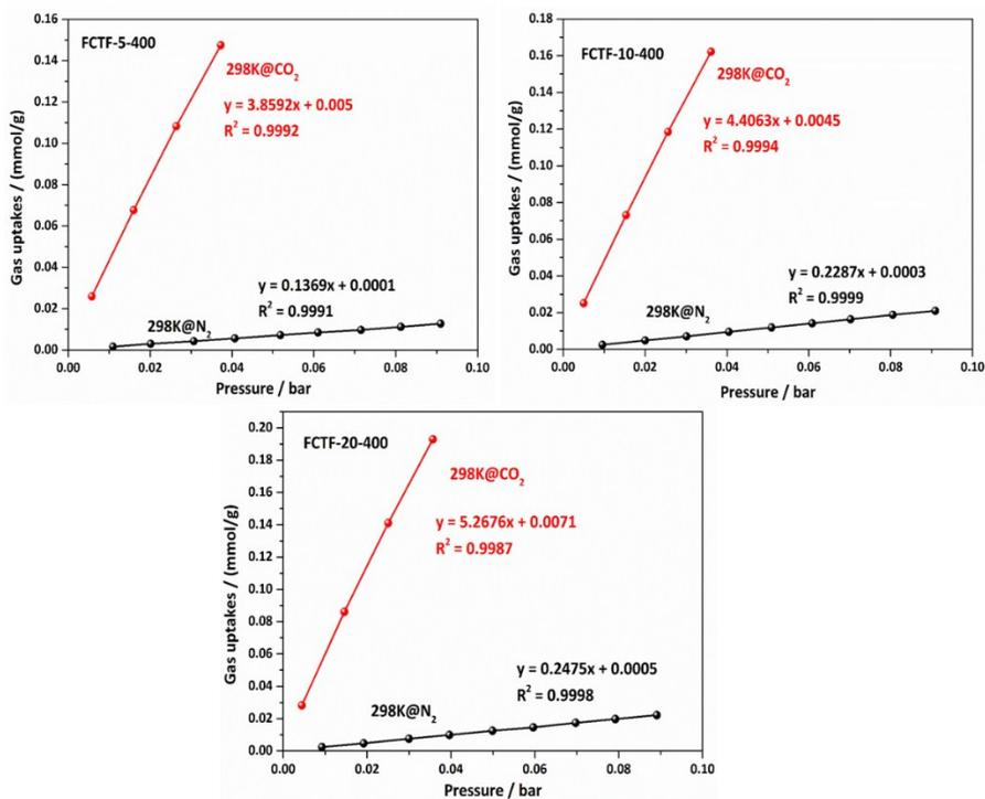
Figure S15. The selectivity of the FCTFs for CO<sub>2</sub> over N<sub>2</sub> isotherms obtained from the initial slope method at 298K.
