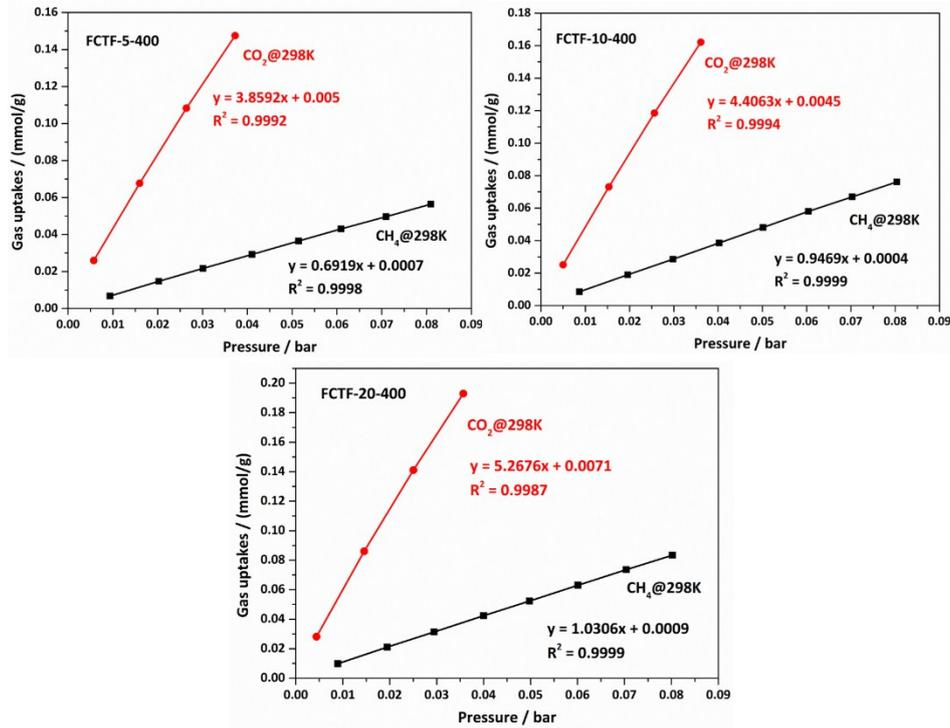
Figure S16. The selectivity of the FCTFs for CO<sub>2</sub> over CH<sub>4</sub> isotherms obtained from the initial slope method at 298K.
