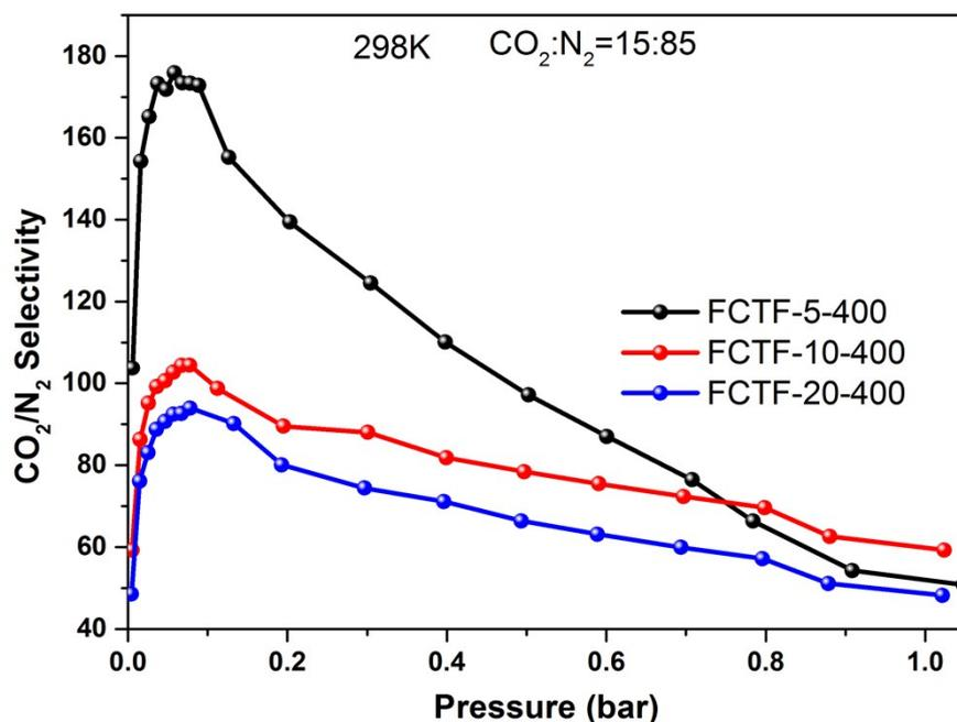
Figure S17. Calculated IAST selectivity of binary gas mixtures ( $\text{CO}_2:\text{N}_2 = 15:85$ ) at 298 K for all the studied FCTFs.
