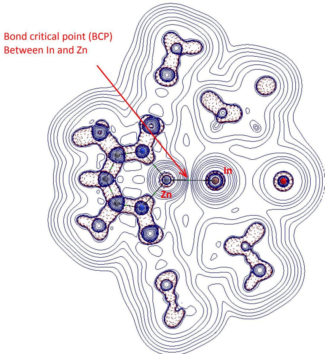
**Figure S27** Molecular graph of  $(\text{NON}^{\text{Dipp}})\text{In}-(\mu\text{-NMes})-\text{Zn}(\text{BDI}^{\text{Mes}})$  (**5**). Solid lines between the atoms are bond paths (very long bond paths are shown with dotted lines). Small green spheres are bond critical points.
