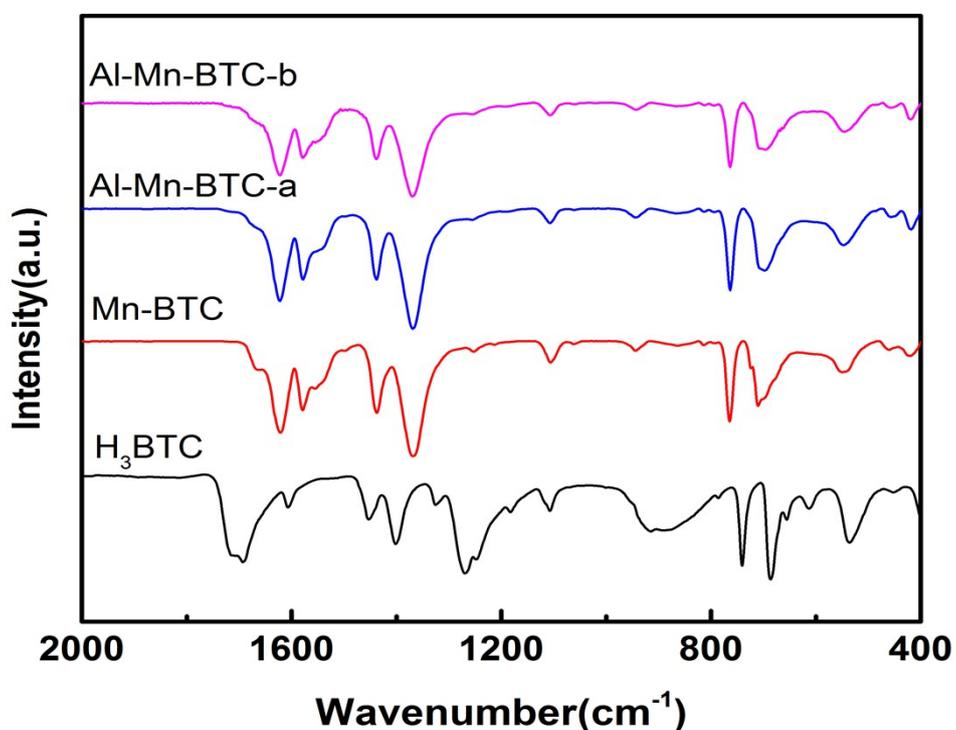
**Fig.S1** FTIR spectra of Mn-BTC, Al-Mn-BTC-a, Al-Mn-BTC-b and H<sub>3</sub>BTC.
