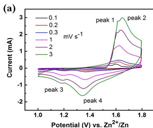
**Fig.S6** (a) CV curves of  $\text{Mn}_2\text{O}_3/\text{Al}_2\text{O}_3\text{-b}$  electrode at different scan rate.
