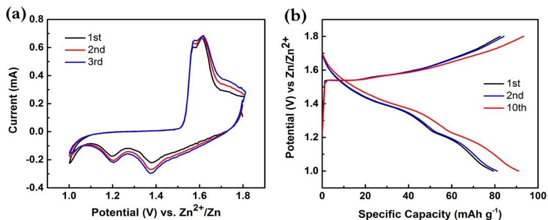
**Fig.S4** Electrochemical performance of the Mn<sub>2</sub>O<sub>3</sub>/Al<sub>2</sub>O<sub>3</sub>-b based AZIB. (a) CV at a scan rate of 0.5 mV·s<sup>-1</sup> in the potential window of 1.0–1.8 V vs. Zn<sup>2+</sup>/Zn.(b) Discharge–charge profile at a current density of 300 mA g<sup>-1</sup>.
