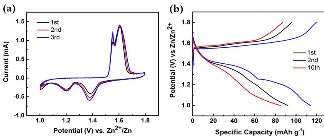
**Fig.S3** Electrochemical performance of the  $\text{Mn}_2\text{O}_3$  based AZIB. (a) CV at a scan rate of  $0.5 \text{ mV} \cdot \text{s}^{-1}$  in the potential window of 1.0–1.8 V vs.  $\text{Zn}^{2+}/\text{Zn}$ . (b) Discharge–charge profile at a current density of  $300 \text{ mA} \cdot \text{g}^{-1}$ .
