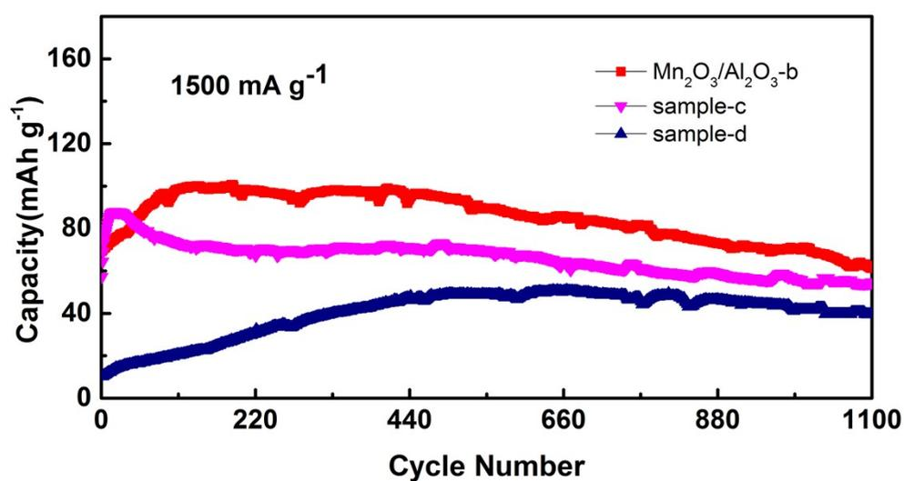
**Fig.S5** Long-term cycling performance of different Al:Mn molar ratio Mn<sub>2</sub>O<sub>3</sub>/Al<sub>2</sub>O<sub>3</sub> electrodes at a high current density of 1500 mA g<sup>-1</sup>.
