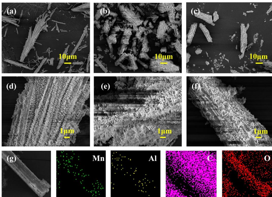
**Fig.S2** The SEM images of Mn-BTC (a, d), Al-Mn-BTC-a (b, e), and Al-Mn-BTC-b (c, f), and the corresponding EDS mapping images of a single Al-Mn-BTC-a nanorod (g).
