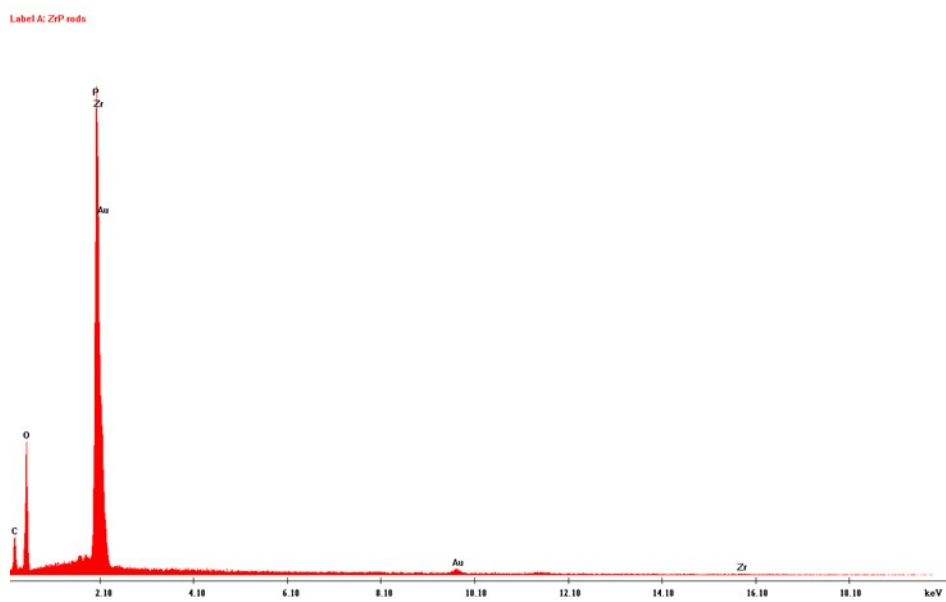
Figure S8. EDS spectrum of \text{ZrP}_{\text{rods}} .
