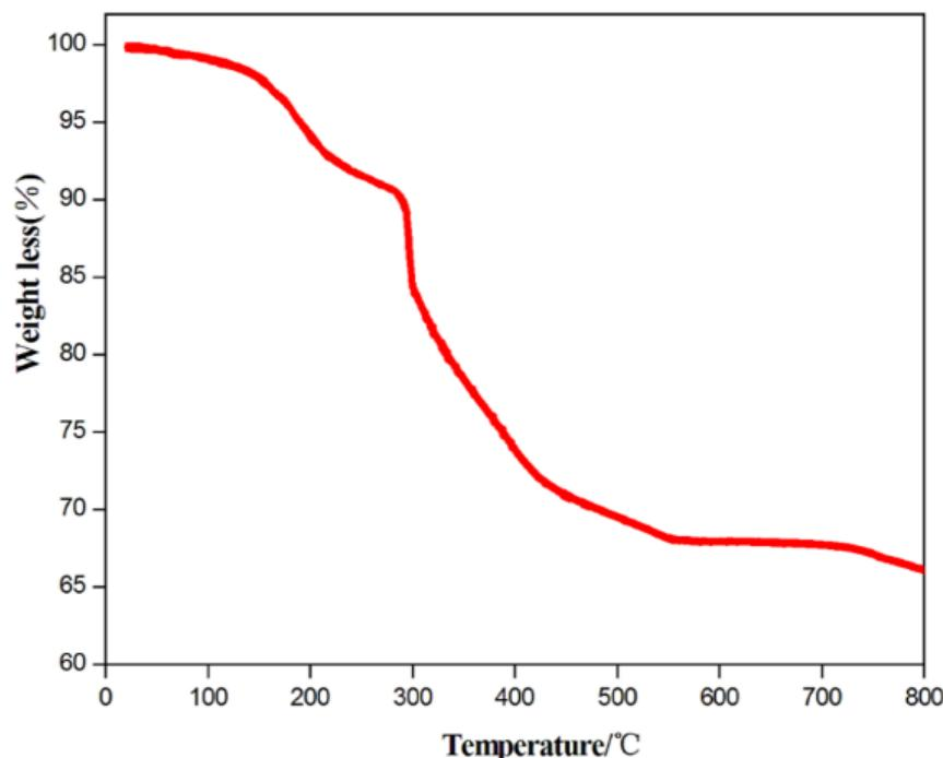
**Figure S7.** The TGA curve (thermal stability) of the porous crystalline POM@MOFs material.
