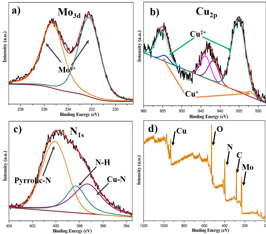
**Figure S8.** High-resolution XPS spectra of Mo (a), Cu (b), N (c) and XPS spectra of the fresh crystalline POM@MOFs material, respectively.
