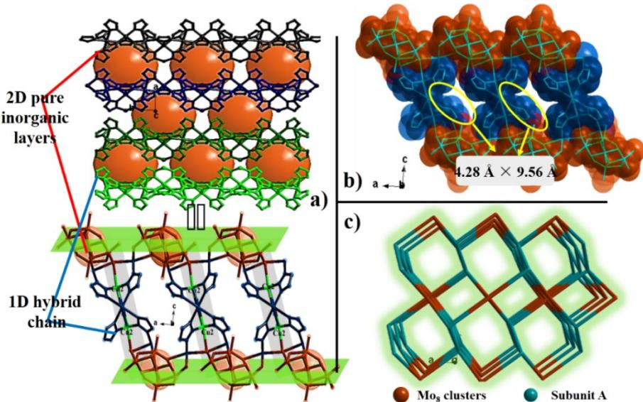
**Figure S3.** Combined ball/stick, stacked and topologic representation of the 3D pillared hybrid frameworks with opening feature formed by 1D hybrid chain and 2D pure inorganic layers in crystalline POM@MOFs.
