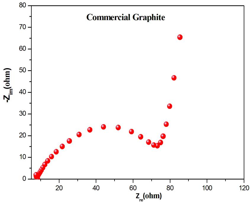
**Figure S5.** Nyquist plots and fitting plots after the first discharge-charge process of commercial graphite anode.
