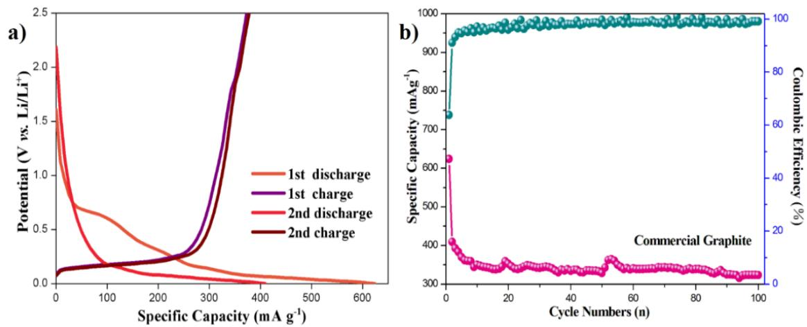
**Figure S4.** The charge-charge curve, cycle stabilities and columbic efficiency of commercial graphite.
