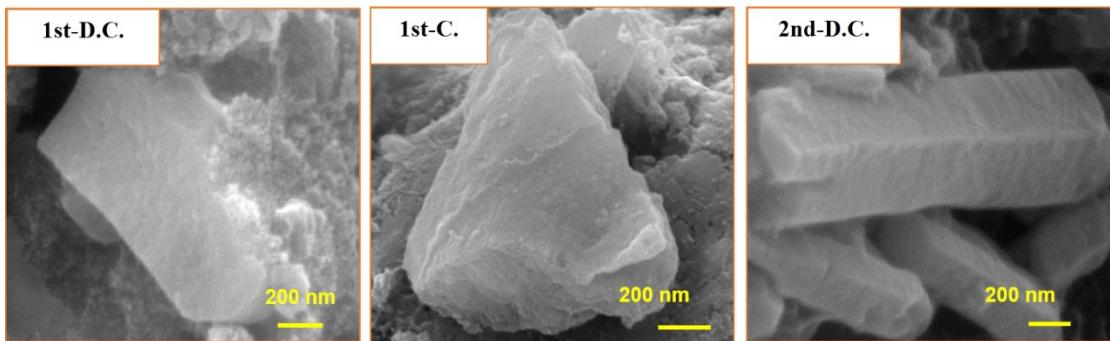
**Figure S9.** SEM images of the crystalline POM@MOFs material after 1st-discharge, 1st-charge and 2nd-discharge, D.C. = discharge, C. = charge.
