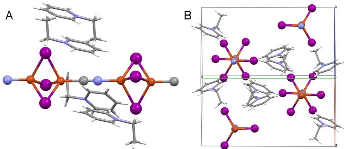
**Figure S2.** X-ray Structure of **4**, anion shown as ball and stick, cation shown as wireframe. A: chain structure with disorder shown in one pair of cations as non-connected atoms; B: unit cell viewed down *a*-axis. Color scheme: orange = Cu, purple = I, grey = C, blue = N.
