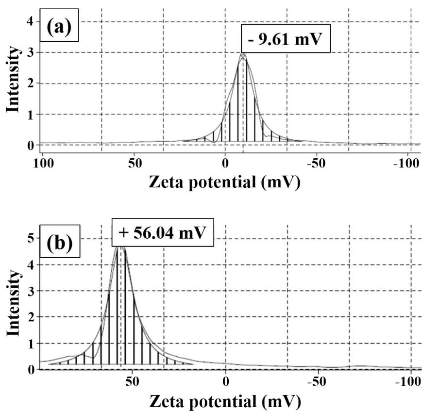
**Fig. S4.** Zeta-potential values of (a) bare Fe<sub>2</sub>O<sub>3</sub>, (b) C-Fe<sub>2</sub>O<sub>3</sub>.
