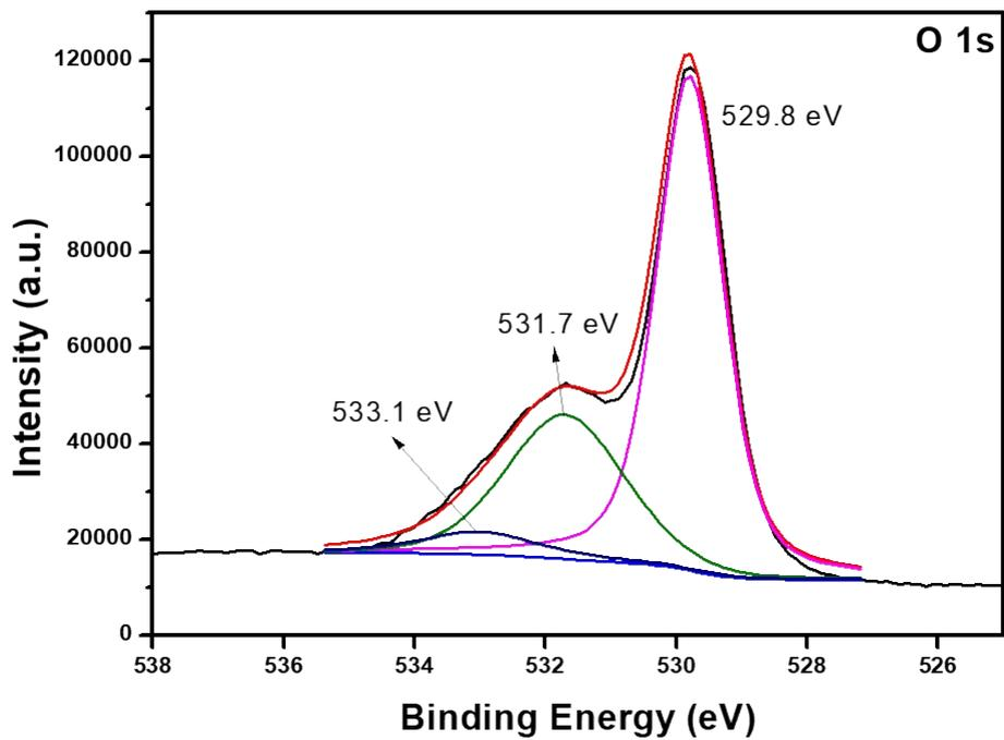
**Fig. S5.** X-Ray photoelectron spectroscopy (XPS) spectra of O 1s in C-Fe<sub>2</sub>O<sub>3</sub>@Au.
