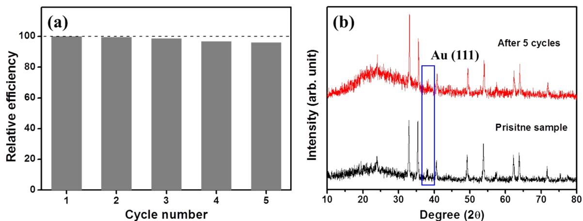
**Fig. S8.** (a) Reusability of  $\text{C-Fe}_2\text{O}_3@\text{Au}$  (0.1 ml) in the photocatalytic degradation of MB, (b) XRD patterns of  $\text{C-Fe}_2\text{O}_3@\text{Au}$  (0.1 ml) before and after the photocatalytic reaction.
