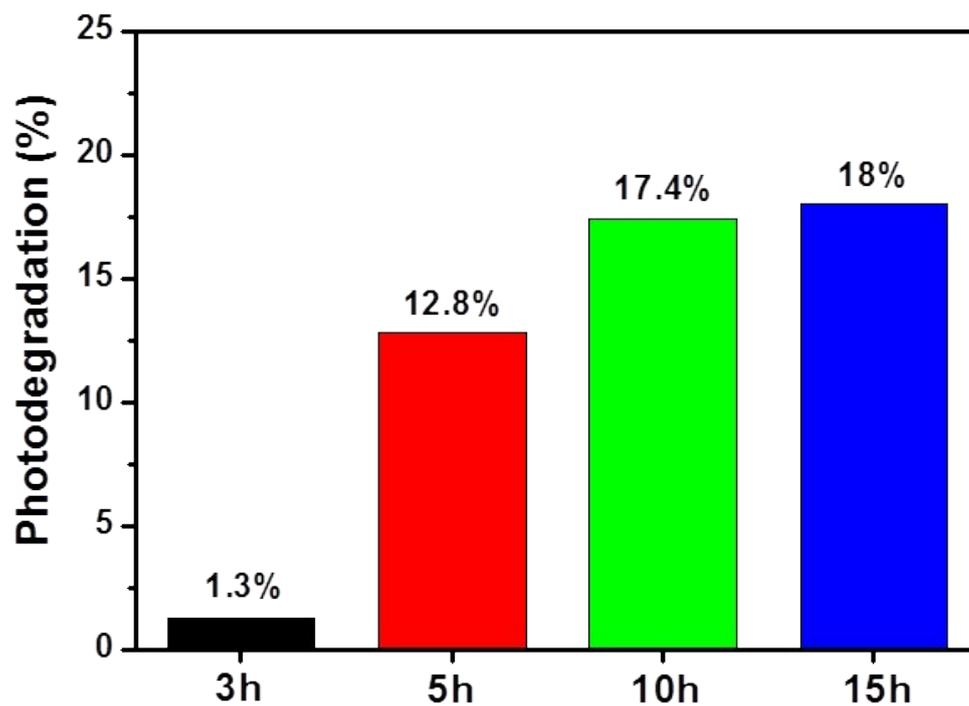
**Fig. S7.** Photodegradation efficiency of methylene blue (MB) over the  $\text{Fe}_2\text{O}_3$  particles prepared at different reaction times (3, 5, 10, and 15 h).
