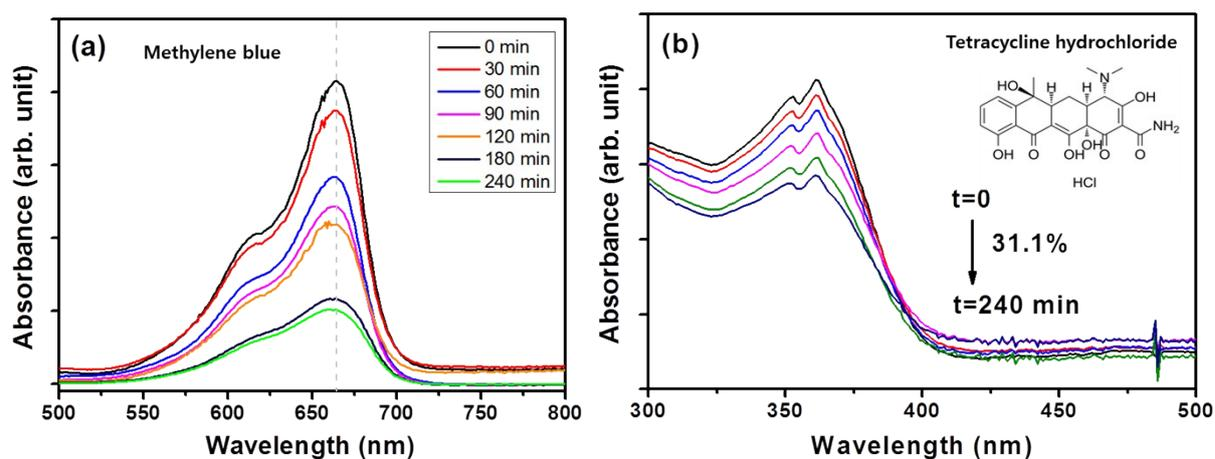
**Fig. S9.** Absorbance changes of organic pollutants over C-Fe<sub>2</sub>O<sub>3</sub>@Au (0.1 ml) during the photodegradation process: a) Methylene blue (10 ppm), b) Tetracycline hydrochloride (5 ppm).
