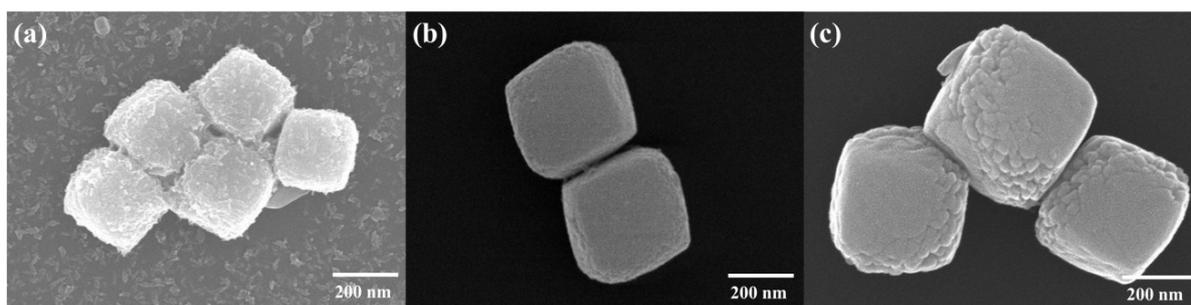
**Fig. S6.** SEM images of C-Fe<sub>2</sub>O<sub>3</sub> prepared at different reaction times: (a) 5 h, (b) 10 h, (c) 15 h.
