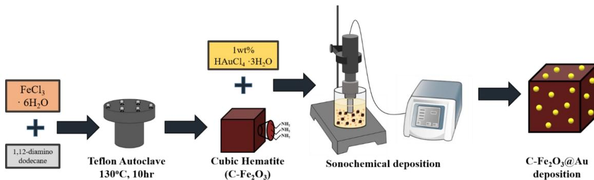
**Fig. S1.** Synthetic procedures of Au-deposited C-Fe<sub>2</sub>O<sub>3</sub> (C-Fe<sub>2</sub>O<sub>3</sub>@Au) through the consecutive hydrothermal and ultrasonic deposition methods.
