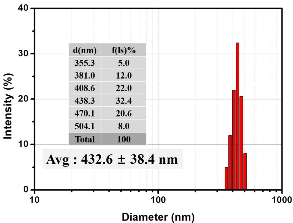
**Fig. S2.** Particle size distribution of C-Fe<sub>2</sub>O<sub>3</sub> by dynamic light scattering (DLS) method.
