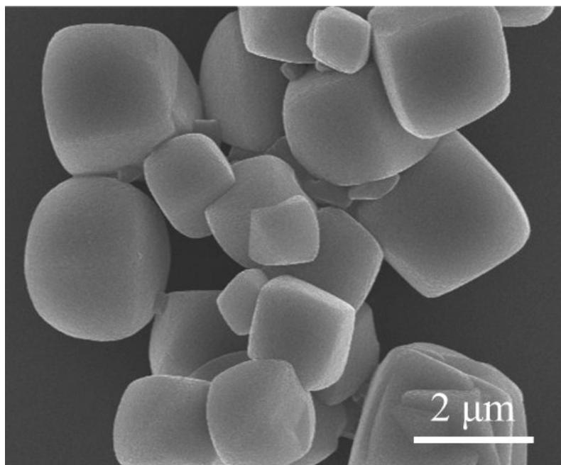
**Fig. S3.** SEM image of bare Fe<sub>2</sub>O<sub>3</sub> prepared without D-12 diamine.
