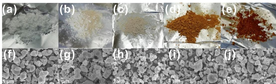
**Fig. S5** Photo pictures and SEM images of ZIF-F before and after thermal treatments under different temperatures for 12 h: (a, f) before heating, (b, g) 200 °C, (c, h) 300 °C,
