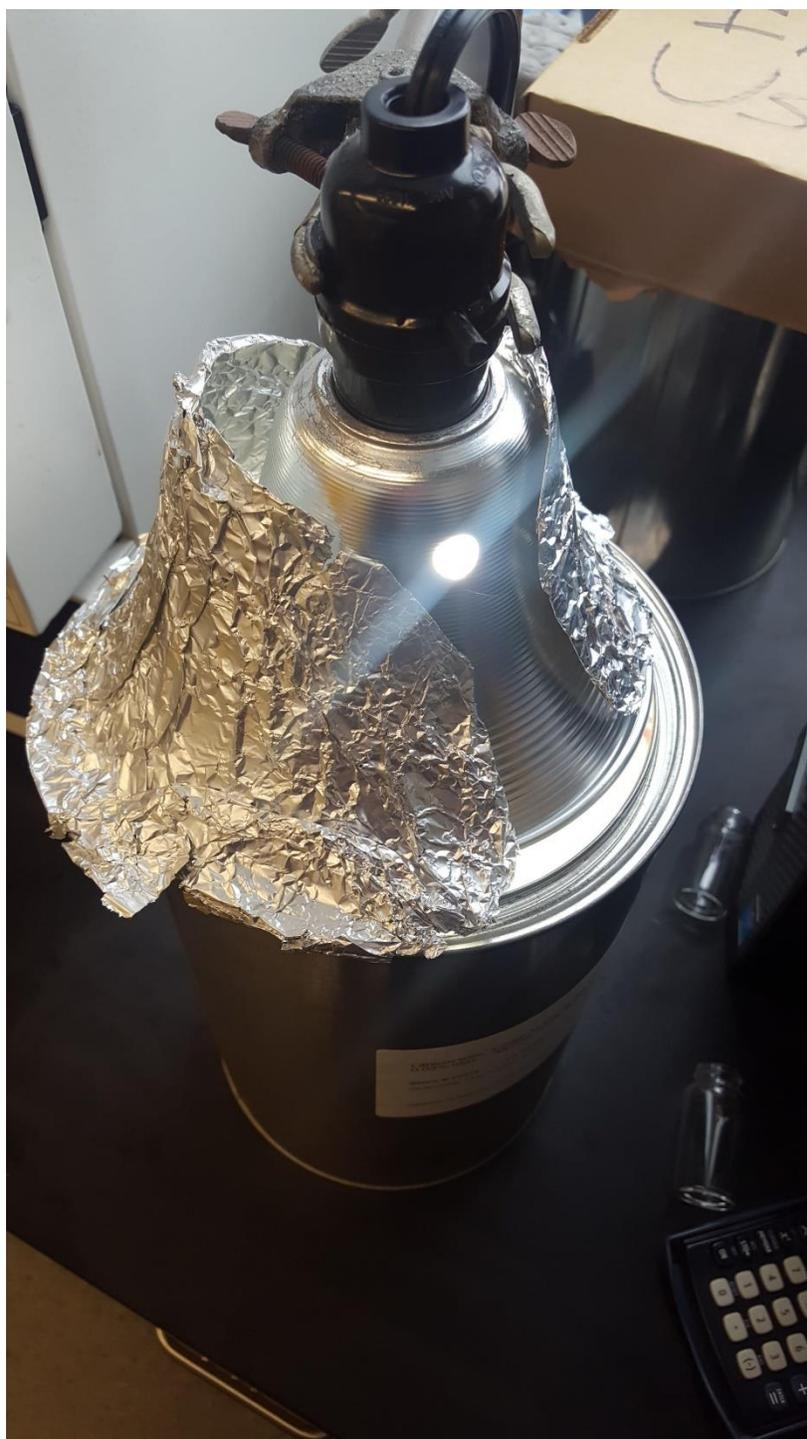
**Figure S.1** LED Reactor for Photocatalysis
