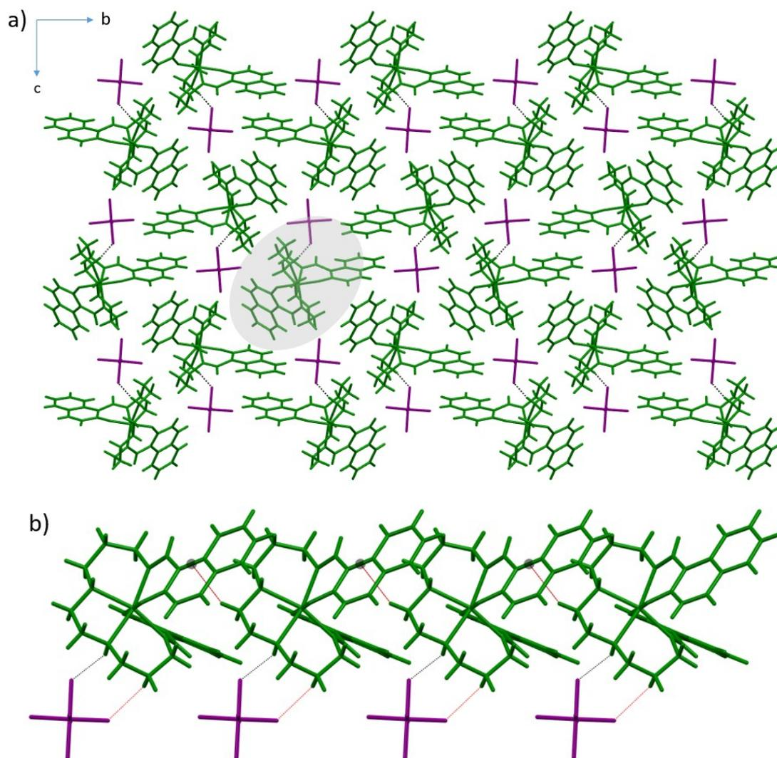
Figure S7. (a) Crystal packing of complex **1** at 295 K, viewed along the *a* axis, showing the N–H···F hydrogen bonds between the [Mn(naphth-sal-N-1,5,8,12)]<sup>+</sup> cations and SbF<sub>6</sub><sup>-</sup> anions. The chain is shown in the light grey background. (b) The chain viewed along the *c* axis. The N–H···F hydrogen bonds are indicated by black dotted lines. The C–H···π and C–H···F hydrogen bonds are indicated by red dotted lines.
