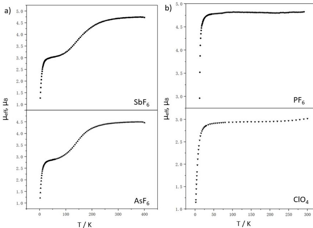
Figure S13. (a) Temperature dependence of the  $\mu_{\text{eff}}$  for [Mn(naphth-sal-N-1,5,8,12)]SbF<sub>6</sub> (**1**) and [Mn(naphth-sal-N-1,5,8,12)]AsF<sub>6</sub> (**2**) between 2–400 K. (b) Temperature dependence of the  $\mu_{\text{eff}}$  for [Mn(naphth-sal-N-1,5,8,12)]PF<sub>6</sub> (**3**) and [Mn(naphth-sal-N-1,5,8,12)]ClO<sub>4</sub> (**4**) between 2–300 K.
