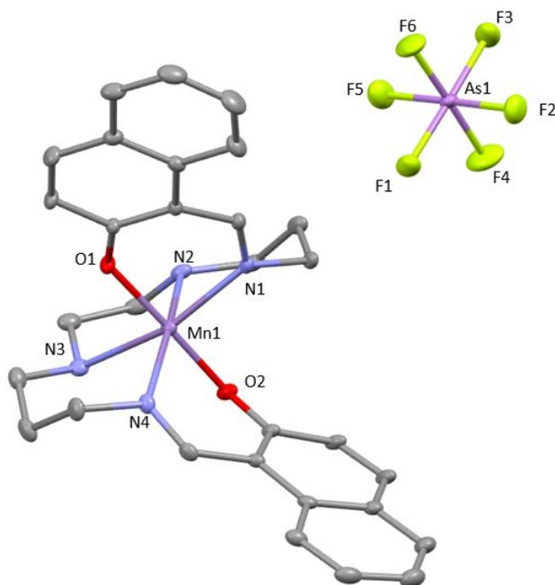
Figure S4. The molecular structure for complex **2** at 295 K, hydrogen atoms have been omitted for clarity.
