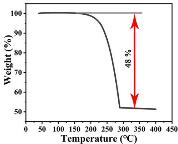
**Fig. S4.** Thermogravimetric curve of curves in air of the NCOHF/S composite.
