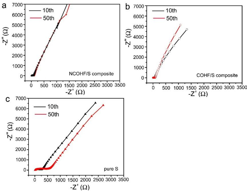
**Fig. S9.** Nyquist plots for NCOHF/S (a), COHF/S (b) and S electrodes (c) after 10<sup>th</sup> and 50<sup>th</sup> cycle.
