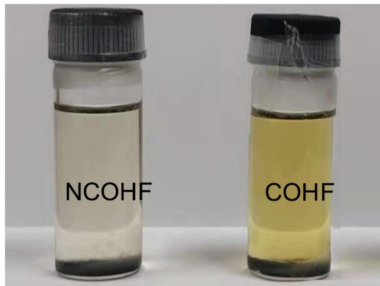
**Fig. S8.** The LiPSSs adsorption ability experiment of NCOHF and COHF: the digital graph of NCOHF and COHF in LiPSSs solution after 4 hours.
