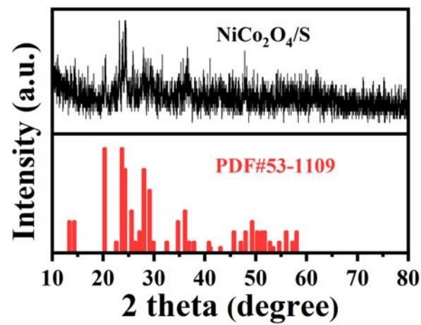
**Fig. S3.** XRD patterns of NCOHF/S composite structures (upper panel) and raw sulfur (lower panel).
