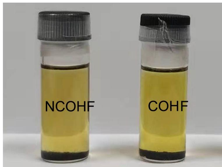
**Fig. S7.** The LiPSSs adsorption ability experiment of NCOHF and COHF: the digital graph of NCOHF and COHF in LiPSSs solution in the beginning.
