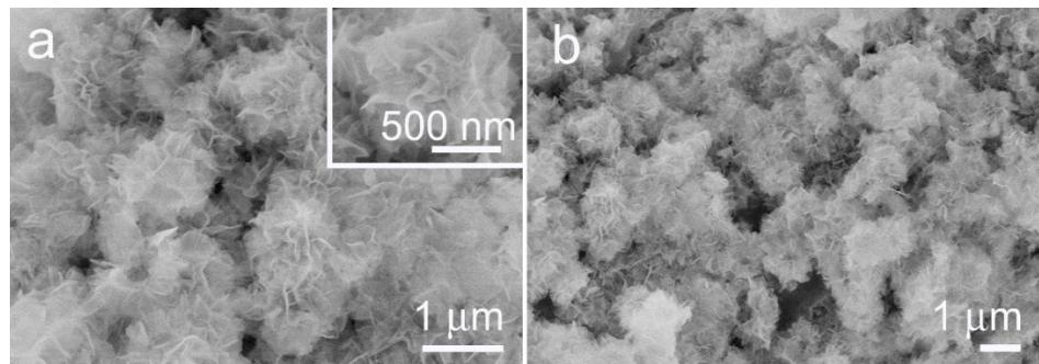
**Fig. S5.** (a) SEM image of Co<sub>3</sub>O<sub>4</sub> hollow nanoflowers (COHF). (b) SEM image of COHF/S composite.
