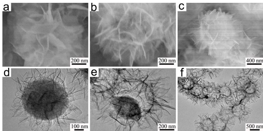
**Fig. S1.** (a-f) SEM morphologies of the precursor of NCOHF taken after reaction for: (a, d) 0.5 h, (b, e) 1 h, (c, f) 3 h, respectively.
