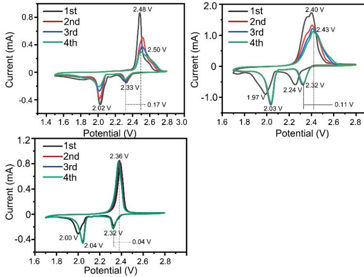
**Fig. S6.** CV profiles of S (a), COHF/S composite (b) and NCOHF/S composite (c)
