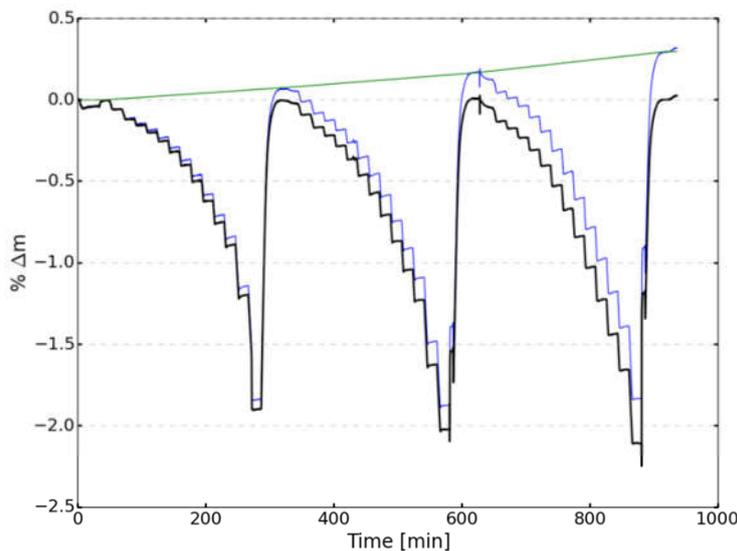
a) The mass change of the redox material is measured in the thermobalance using different temperatures and oxygen partial pressures. Different temperature and pressure programs are chosen to match the expected conditions in which the redox material is most active. One of these measurements is shown here, but up to three measurements per material are combined to get one thermodynamic dataset.
