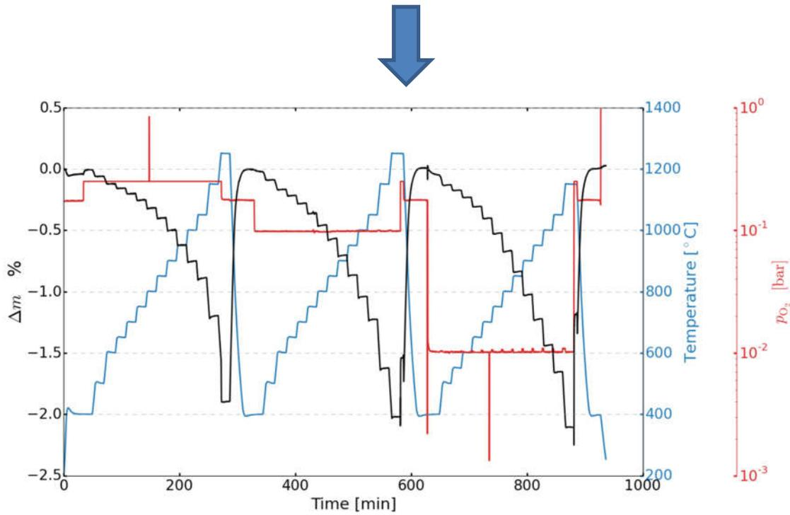
c) The corrected data (black) can then be shown together with the pressure data (red) from the lambda sensor. Short-term spikes in pressure are artefacts of the sensor which are ignored. Please note that the pressure sensor can only measure partial pressures up to 0.25 bar O<sub>2</sub>.
