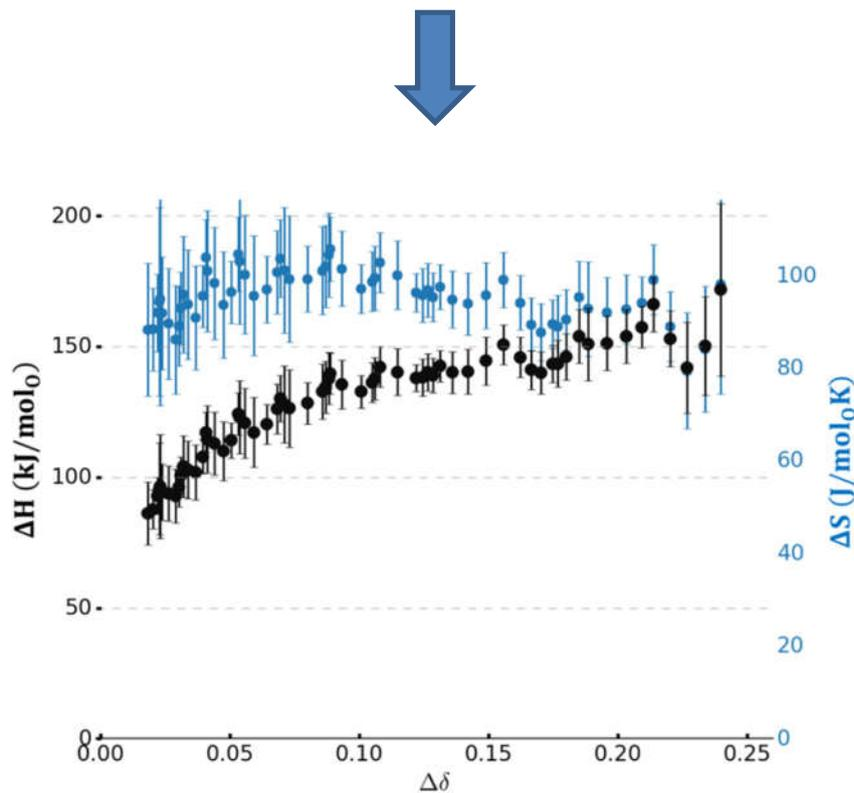
f) The enthalpy and entropy change as a function of  $\Delta\delta$  per mol of oxygen O can then be shown in a new plot. The measurement uncertainties are derived as the square roots of the covariance matrices of the linear fits in the previous plot.
