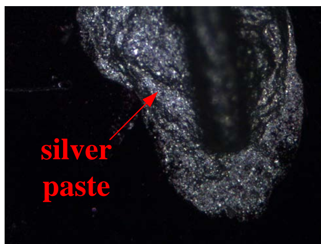
Figure S16. Prototype schematic diagram for Raman scattering spectra experiment of the BCT-BMT thin film under dc bias electric field. (a) Sample bridged by silver paste rather than by the wire bonding method to minimize damage. Optical microscope images of the ITO top electrode under bright field (b) and dark field (c).
