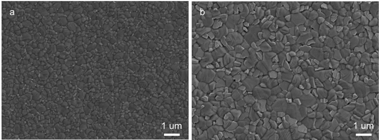
**Fig. S12. SEM top-view images of the perovskite films with one-step (a) and two-step method (b).**
