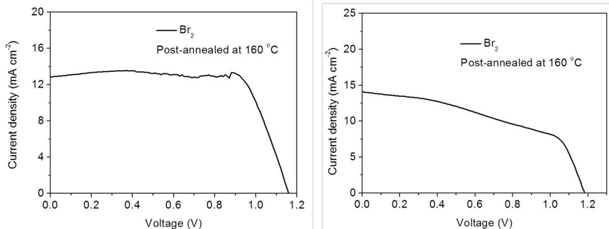
**Fig. S8. Typical  $J$ - $V$  curves of perovskite solar cells with c-TiO<sub>2</sub>/Br<sub>2</sub> electron transporting layers prepared at 160 °C.**
