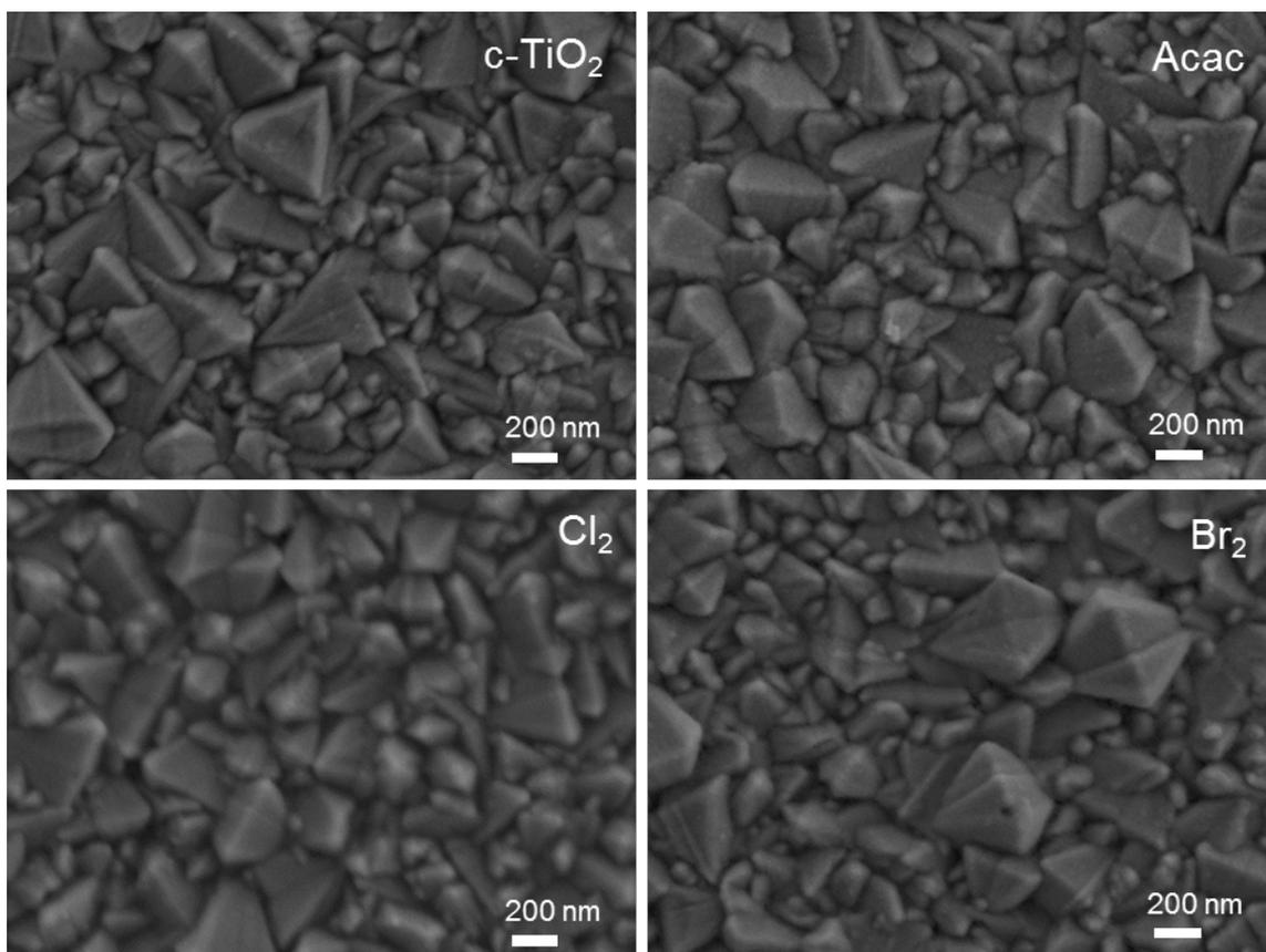
**Fig. S6. Top-view images SEM of c-TiO<sub>2</sub>, Acac, Cl<sub>2</sub> and Br<sub>2</sub> on FTO, respectively, taken at a small area. Films are annealed at 180 °C 1 h.**
