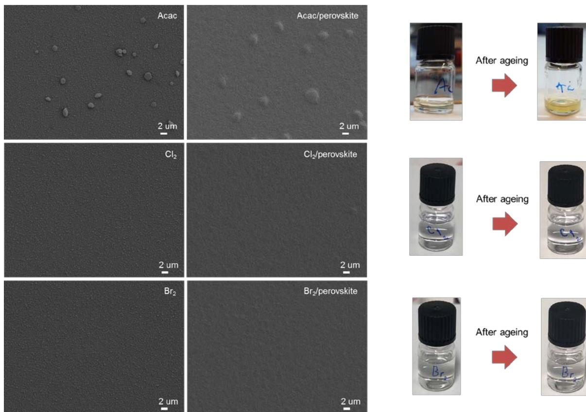
**Fig. S7. Top-view SEM images of Acac, Cl<sub>2</sub> and Br<sub>2</sub> films on FTO/c-TiO<sub>2</sub> substrates (left), and perovskite top-surface images on each ETL. An Acac solution in DMF turns into a turbid solution in a few hours while solutions show no color or transparency change.**
