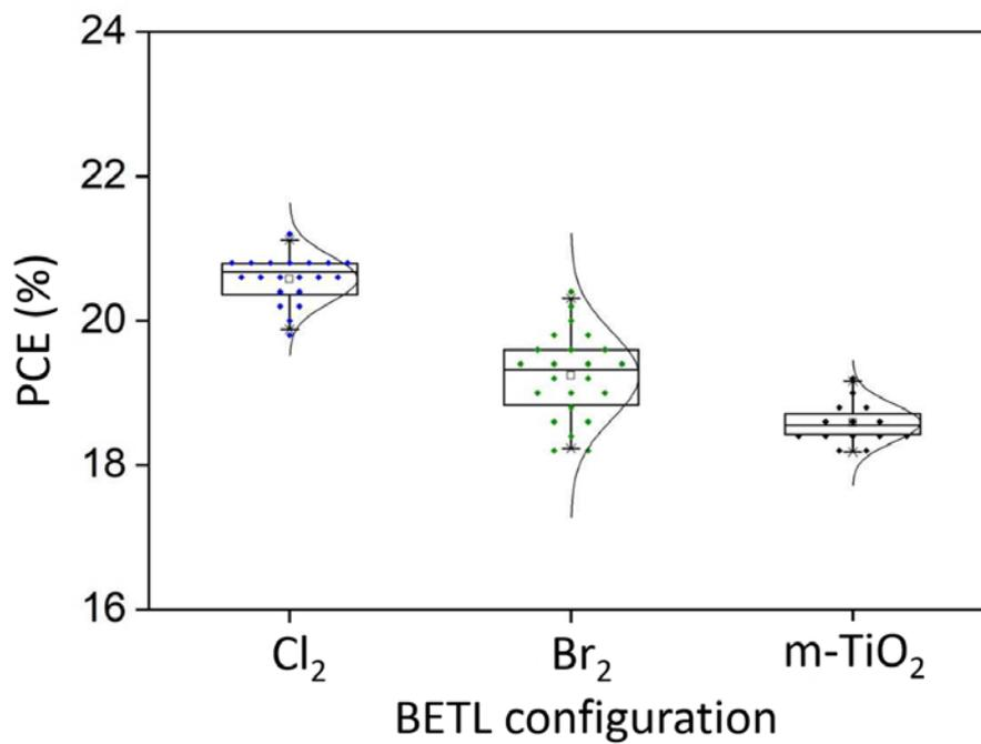
**Fig. S15.** Box plot for device PCE for Cl<sub>2</sub>, Br<sub>2</sub> and m-TiO<sub>2</sub> BETL configurations.
