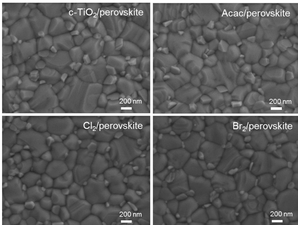
**Fig. S5. Top-view SEM images of the perovskite films formed on c-TiO<sub>2</sub>, Acac, Cl<sub>2</sub> and Br<sub>2</sub> films, respectively.**
