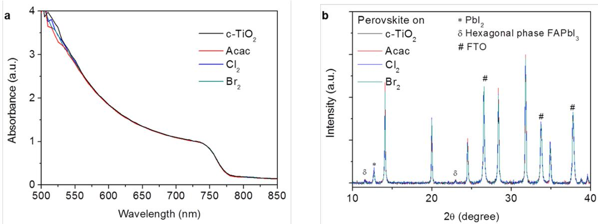
**Fig. S4. Absorbance (a) and XRD patterns (b) of the perovskite film on the FTO/ETLs.**
