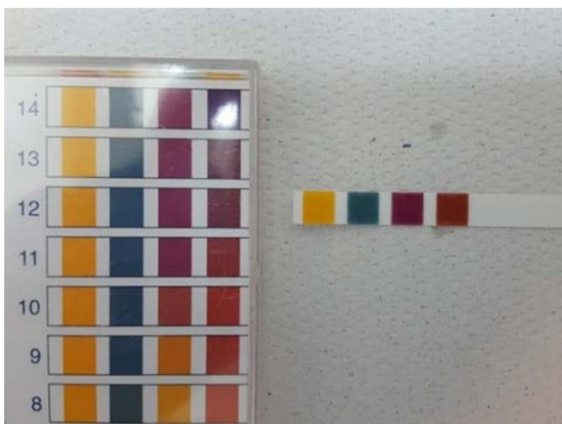
**Fig. S9. pH test of the colloidal SnO<sub>2</sub> 15% in water (AlfaAesar).** The result indicates the colloidal solution is in a highly basic condition with pH=11~12.
