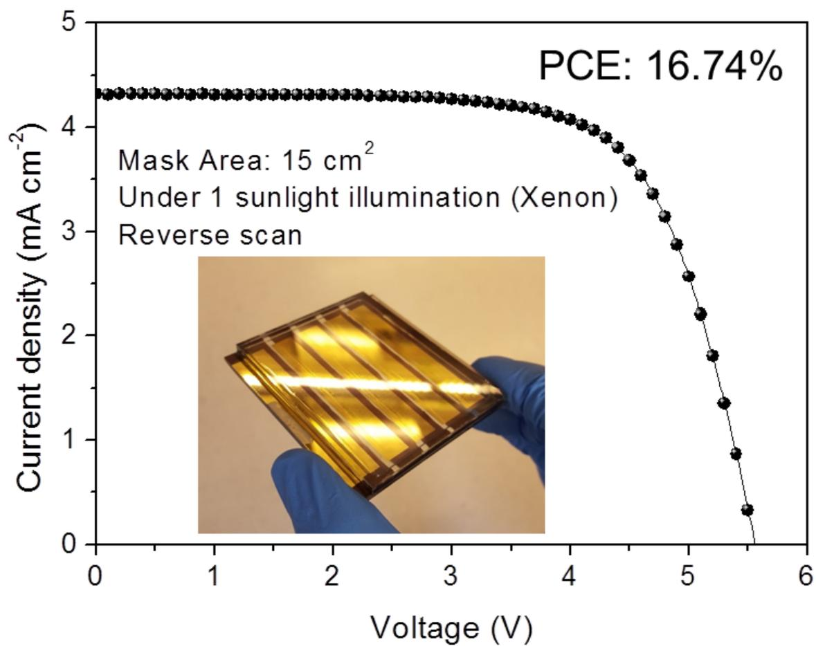
**Fig. S10.** A *J-V* curve of the planar-type perovskite mini-module.
