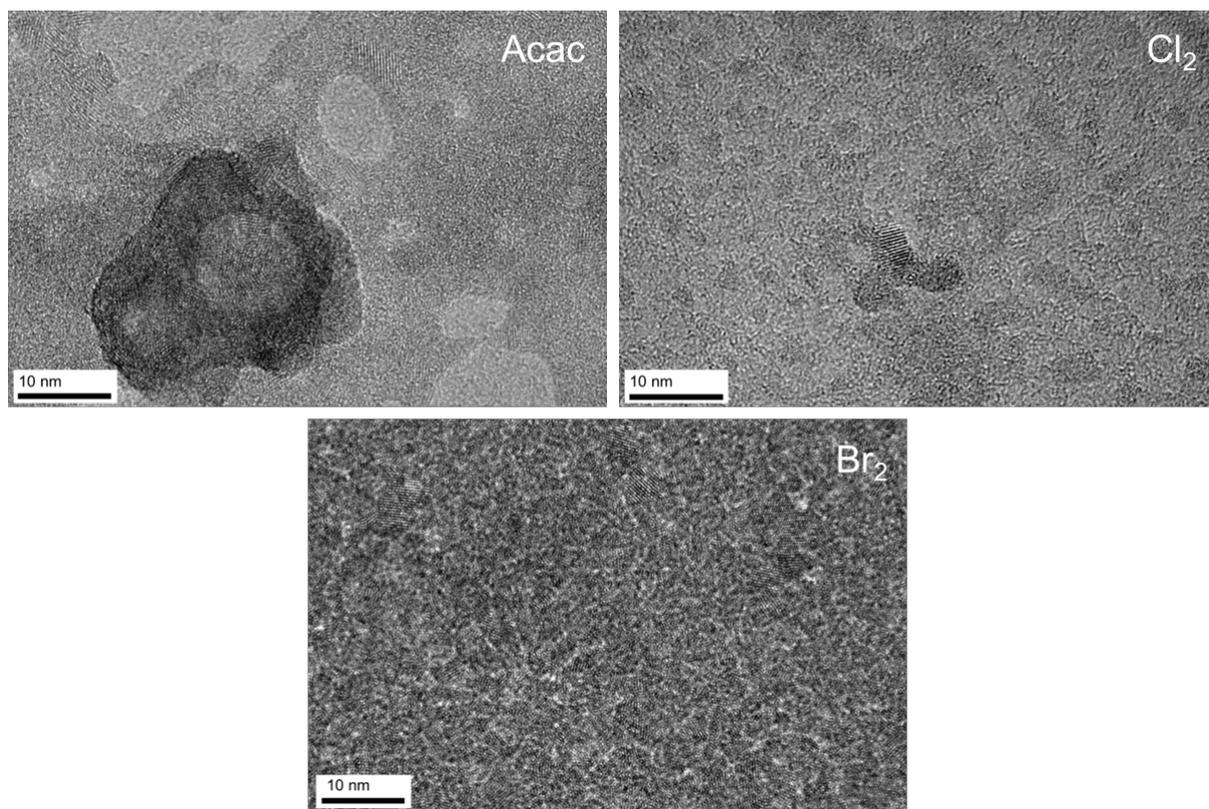
**Fig. S2. HR-TEM images of Acac, Cl<sub>2</sub> and Br<sub>2</sub> annealed at 180 °C.**
