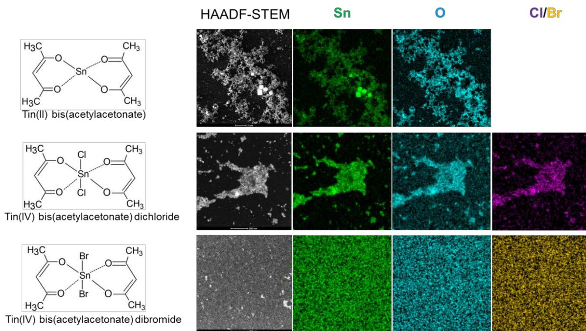
**Fig. S1. EDXS-STEM analysis.** HAADF scanning TEM images and corresponding elemental mapping of Sn, O, Cl and Br of the tin oxide films deposited on a carbon support grid.
