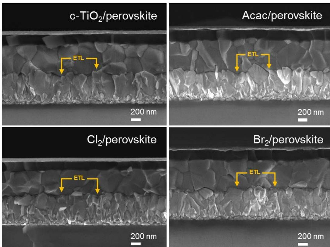
**Fig. S3. SEM cross-sectional images for the complete cells.** The thickness of the ETL layer is higher for Cl<sub>2</sub>/Perovskite and Br<sub>2</sub>/perovskite than Acac/perovskite and c-TiO<sub>2</sub>/perovskite.
