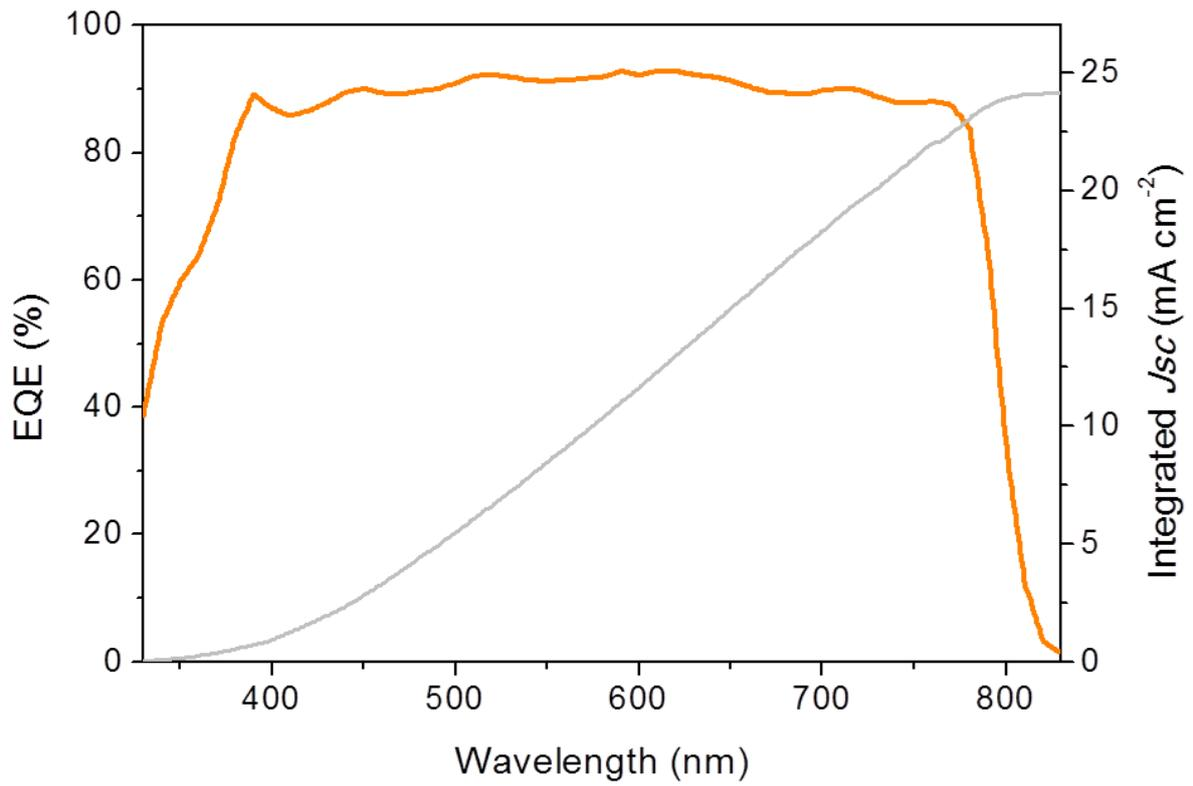
**Fig. S11. External quantum efficiency (EQE) of the champion cell.**
