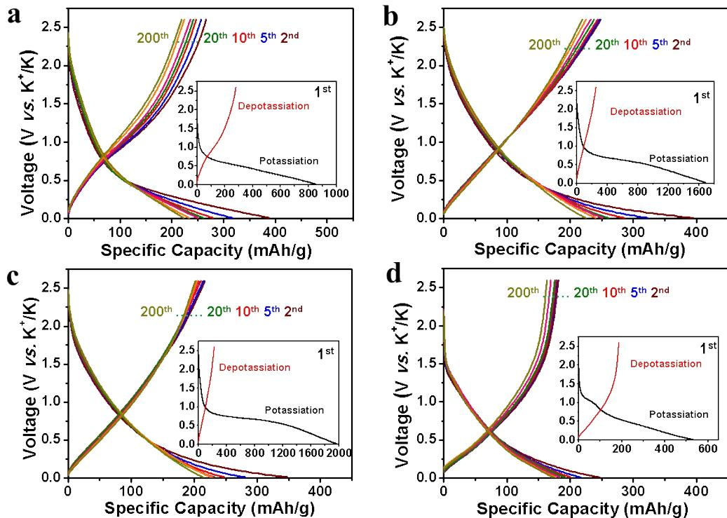
**Figure S12.** The 2<sup>nd</sup>, 5<sup>th</sup>, 10<sup>th</sup>, 20<sup>th</sup>, 50<sup>th</sup>, 100<sup>th</sup> and 200<sup>th</sup> potassiation and depotassiation profiles of the series of NHCFs materials at the current density of 100 mA/g: (a) NHC<sub>1</sub>-NH<sub>3</sub>/Ar, (b) NHC<sub>2</sub>-Ar-800, (c) NHC<sub>2</sub>-Ar-900 and (d) PAN-NH<sub>3</sub>/Ar.
