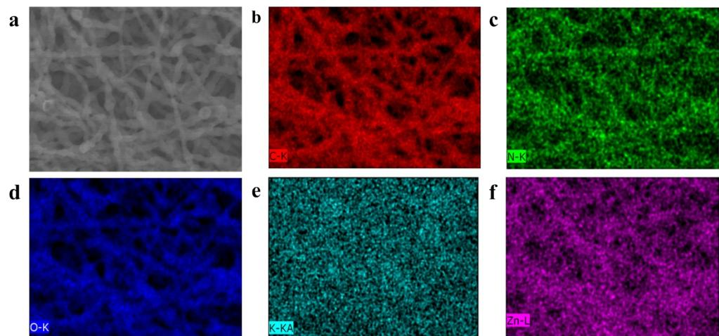
**Figure S18.** (a) SEM image and (b-f) the EDS mappings of the  $\text{NHC}_2\text{-NH}_3/\text{Ar}$  electrode after 100 cycles.
