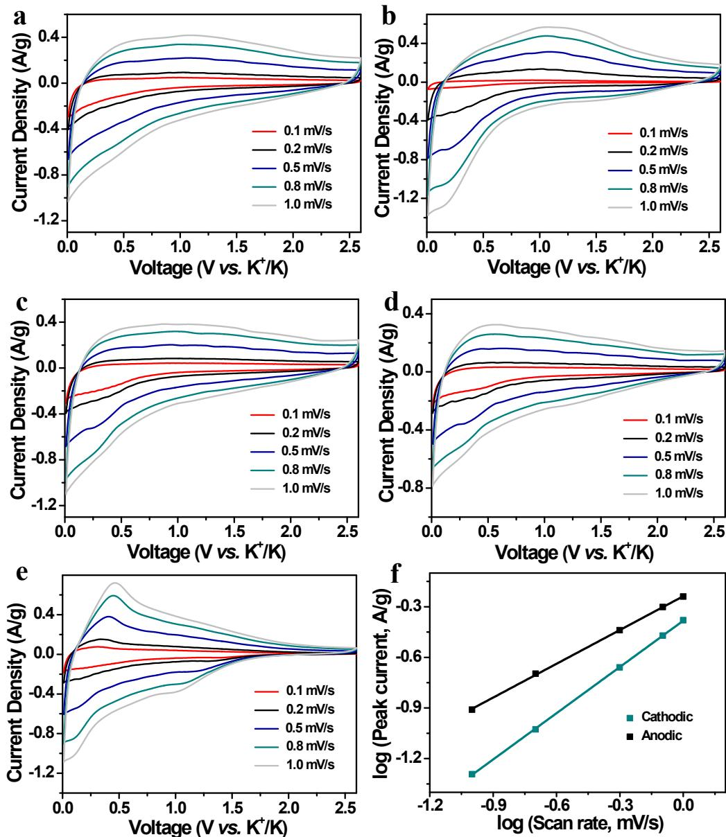
**Figure S20** CV profiles of the series of NHCFs materials at different scan rates: (a) NHC<sub>2</sub>-NH<sub>3</sub>/Ar, (b) NHC<sub>1</sub>-NH<sub>3</sub>/Ar, (c) NHC<sub>2</sub>-Ar-800, (d) NHC<sub>2</sub>-Ar-900 and (e) PAN-NH<sub>3</sub>/Ar. (f) Determination of the b-value of NHC<sub>2</sub>-NH<sub>3</sub>/Ar using the relationship between peak current and scan rate in PIBs.
