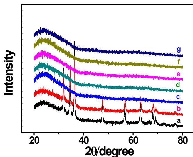
**Figure S5** XRD patterns of the NHC materials: a (NHC<sub>2</sub>-Ar-600), b (NHC<sub>2</sub>-Ar-700), c (NHC<sub>2</sub>-Ar-800), d (NHC<sub>2</sub>-Ar-900), e (NHC<sub>1/2</sub>-NH<sub>3</sub>/Ar), f (NHC<sub>1</sub>-NH<sub>3</sub>/Ar) and g (NHC<sub>2</sub>-NH<sub>3</sub>/Ar).
