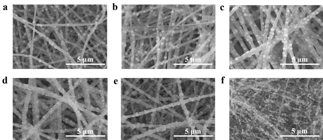
**Figure S2** SEM images of *u*-NHC<sub>x/y</sub> made with different precursor proportions (ZnO:PAN): (a) 1:3, (b) 1:2, (c) 2:3, (d) 1:1, (e) 2:1 and (f) 3:1.
