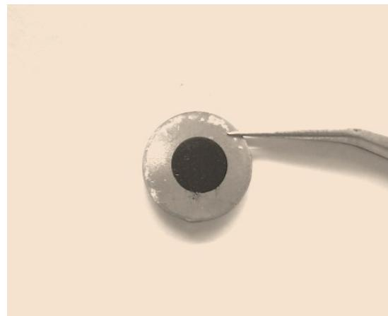
**Figure S16.** Digital photograph of  $\text{NHC}_2\text{-NH}_3/\text{Ar}$  electrode after 1000 cycles
