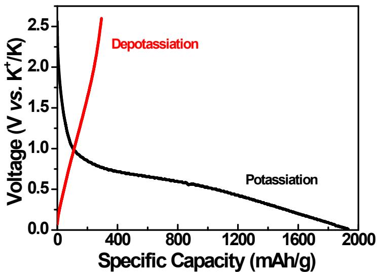
**Figure S11.** Potassiation and depotassiation profiles of the  $\text{NHC}_2\text{-NH}_3/\text{Ar}$  electrode for the first cycle at 100 mA/g.
