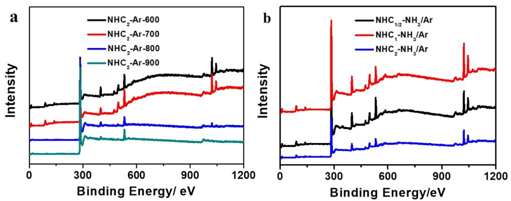
**Figure S6** XPS spectra of different NHC materials.
