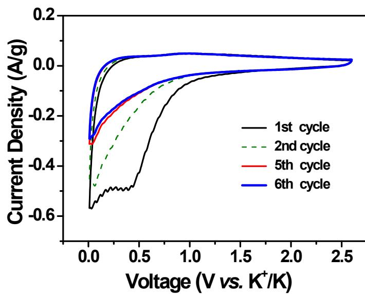
**Figure S13.** Cyclic voltammetry (CV) of the NHC<sub>2</sub>-NH<sub>3</sub>/Ar electrode for PIBs between 0.01 V and 2.5 V with a scan rate of 0.1 mV/s.
