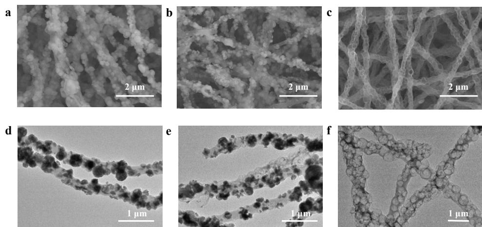
**Figure S4** (a-c) SEM and (d-f) TEM images of NHC pyrolyzed at different temperature in Ar atmosphere: (a, d) NHC<sub>2</sub>-Ar-600, (b, e) NHC<sub>2</sub>-Ar-700 and (c, f) NHC<sub>2</sub>-Ar-800.
