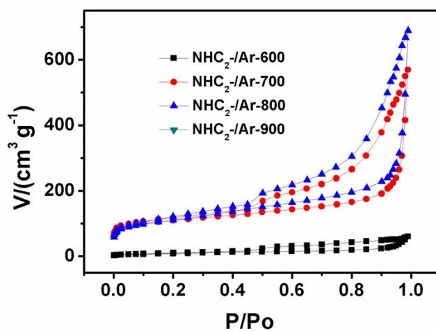
**Figure S8** Nitrogen adsorption-desorption isotherms of the NHC materials.
