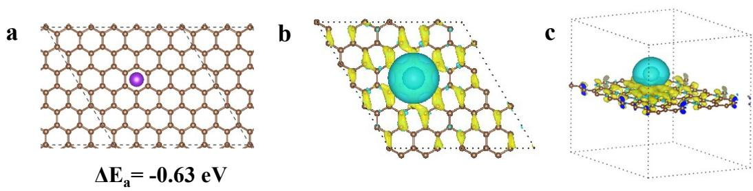
**Figure S21** Theoretical simulations and relative verifications. (a) K atom was absorbed in the pristine carbon structure. Side and top views of electron density differences of K absorbed in the pristine carbon structures. Yellow and blue areas represent increased and decreased electron density, respectively. Brown and purple balls represent C and K atoms, respectively
