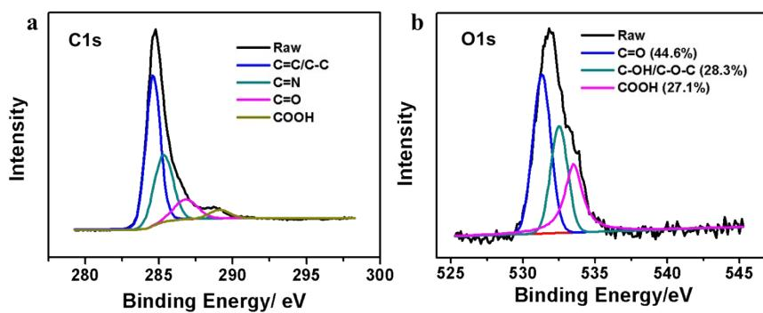
**Figure S7** High-resolution XPS spectra of  $\text{NHC}_2\text{-NH}_3/\text{Ar}$ . (a)  $\text{C}_{1s}$  and (b)  $\text{O}_{1s}$ .
