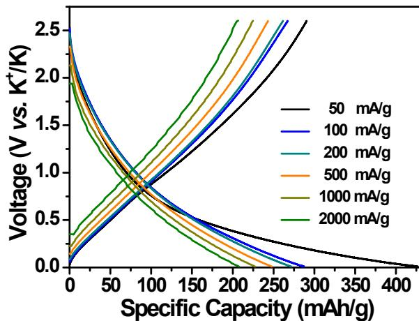
**Figure S14.** The potassiation and depotassiation profiles of the  $\text{NHC}_2\text{-NH}_3/\text{Ar}$  electrode at different current densities from 50 to 2000 mA/g.
