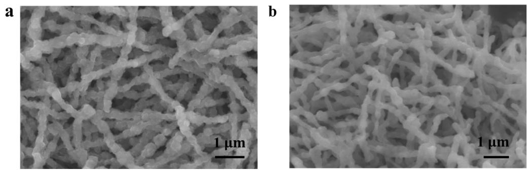
**Figure S17.** SEM images of the  $\text{NHC}_2\text{-NH}_3/\text{Ar}$  electrode after (a) 100 and (b) 1000 cycles.
