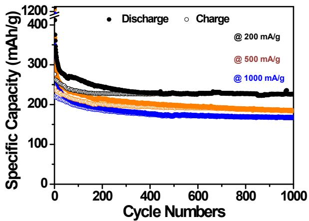
**Figure S15.** The cycles of the  $\text{NHC}_2\text{-NH}_3/\text{Ar}$  electrode measured under different current densities of 200, 500 and 1000 mA/g.
