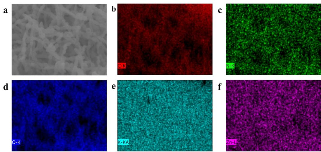
**Figure S19.** (a) SEM image and (b-f) the EDS mappings of the  $\text{NHC}_2\text{-NH}_3/\text{Ar}$  electrode after 1000 cycles.
