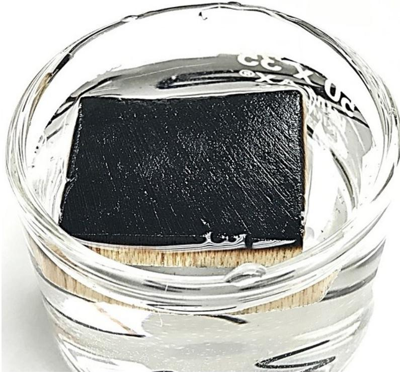
**Figure S10.** The bimodal evaporator can float on brine or sea, which indicates this eco-friendly evaporator can help protect agricultural land and natural ecosystem from being utilized for energy-water nexus.
