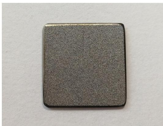
**Fig. S5** Photo of the porous Ti sheet, used as the anode GDL in this work.
