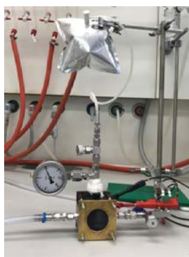
Figure S4. Newly designed pressurised cell for exemplary analysis of the gaseous phase.
