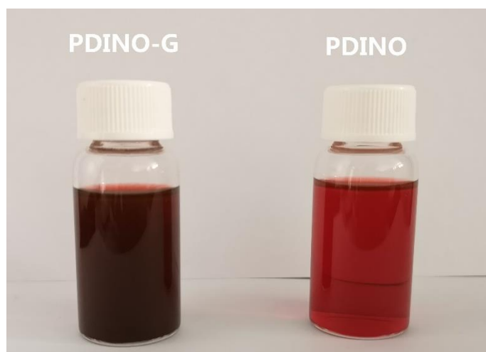
Fig. S2 Photograph of PDINO-G dispersion ( 2 \text{ mg mL}^{-1} PDINO with 5% graphene) and PDINO solution ( 2 \text{ mg mL}^{-1} ).
