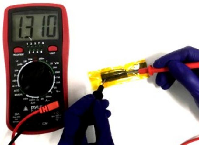
**Figure S29.** The open-circuit potential (OCP) of the flexible rechargeable ZAB.
