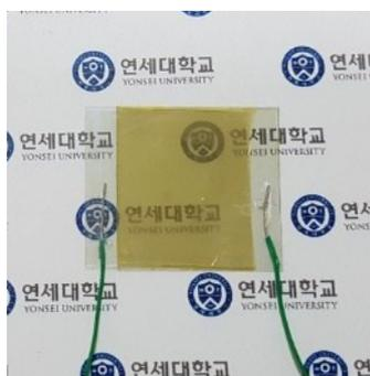
**Fig. S9** A photograph of the CsPbBr<sub>3</sub> thin film-based energy harvester.
