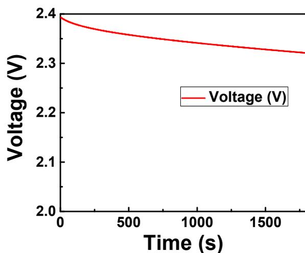
Figure S3. Self-discharge characteristic of the 0.01 F supercapacitor after charged to 2.4 V.
