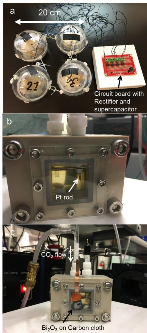
**Figure S2.** Optical images of the (a) spherical TENGs with the charge storage circuit board, electrochemical cell for (b) OER and (c) CO<sub>2</sub>RR.
