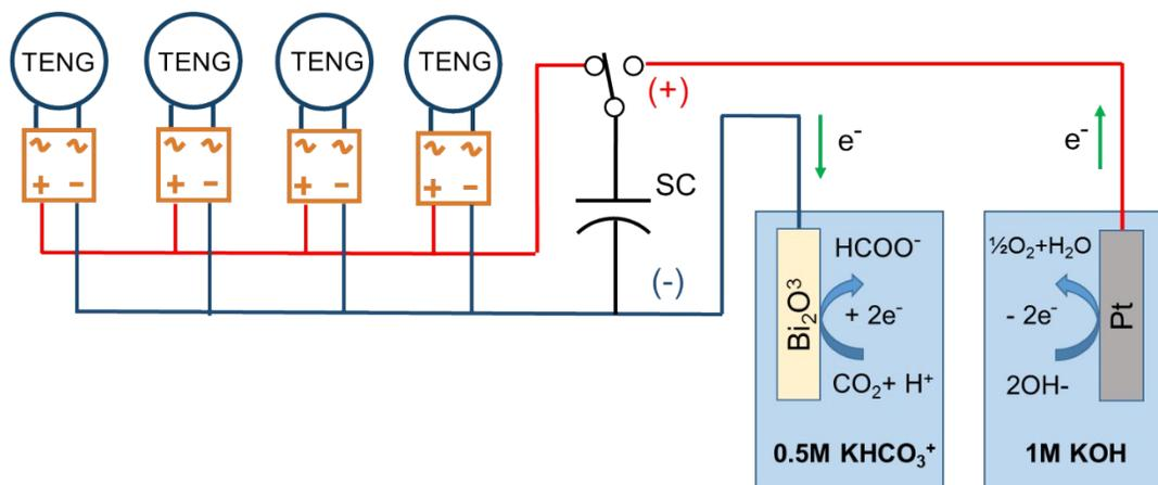
**Figure S1.** Detailed schematic diagram of the wave energy-driven CO<sub>2</sub>RR system
