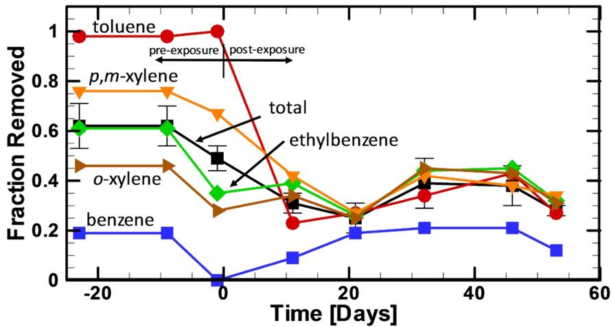
**Figure SI.2.** Average fraction of benzene, toluene, ethylbenzene, *p,m*-xylene, *o*-xylene and total BTEX removed from the three persulfate (PS) bioreactors over the monitoring period. The bioreactors were exposed to the persulfate solution (20 g/L) on Day 0.
