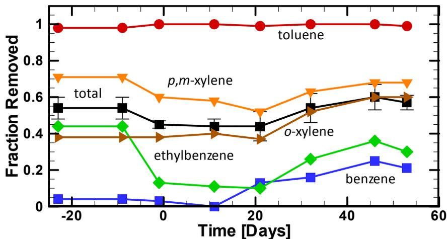
**Figure SI.1.** Average fraction of benzene, toluene, ethylbenzene, *p,m*-xylene, *o*-xylene and total BTEX removed from the three control (CTRL) bioreactors over the monitoring period.
