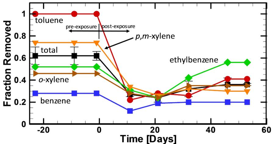
**Figure SI.3.** Average fraction of benzene, toluene, ethylbenzene, *p,m*-xylene, *o*-xylene and total BTEX removed from the three alkaline activated persulfate (ALK-PS) bioreactors over the monitoring period. The bioreactors were exposed to the alkaline activated persulfate solution (20 g/L; pH 12) on Day 0.
