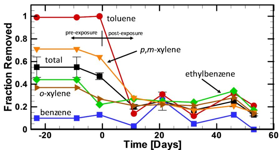
**Figure SI.4.** Average fraction of benzene, toluene, ethylbenzene, *p,m*-xylene, *o*-xylene and total BTEX removed from the three alkaline activated (ALK) bioreactors over the monitoring period. The bioreactors were exposed to the alkaline solution (pH 12) on Day 0.
