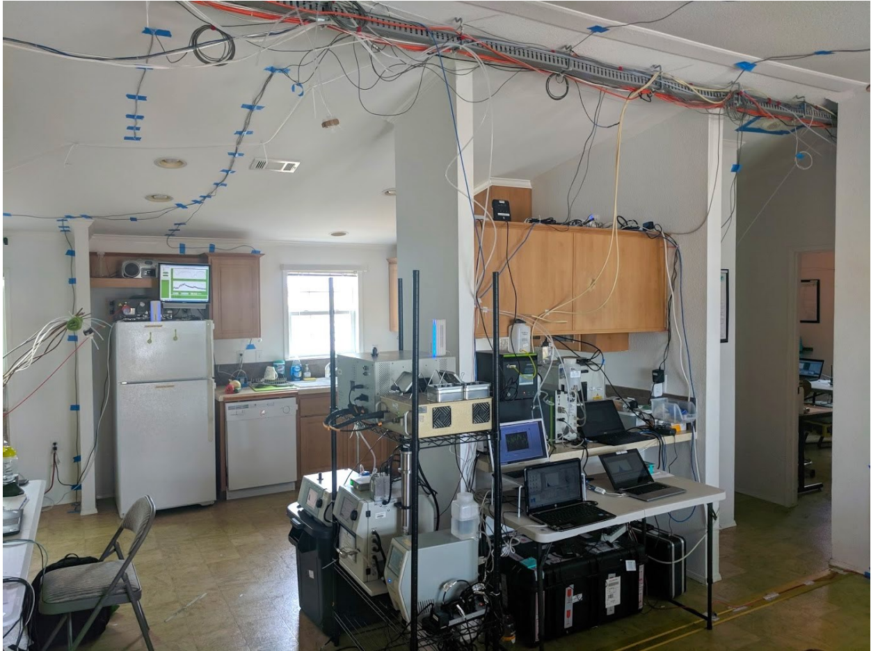
Figure S1. View of open kitchen area with main inlet line for most trace gas and particle measurements near the refrigerator. Inlets were insulated between house and instrument trailers. The dishwasher and sink are apparent in the kitchen. Aerosol size distribution instruments are located on the shelves and kitchen counters. Low-cost sensors and a Portable Optical Particle Sensors (POPS, Table 4) are located on the top of the kitchen cabinets between the kitchen and living space.
