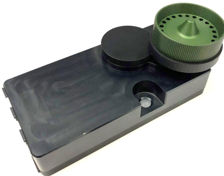
**Fig. S2** A photograph of the MARS with a 1 L·min<sup>-1</sup> cyclone attached via a plastic adapter.
