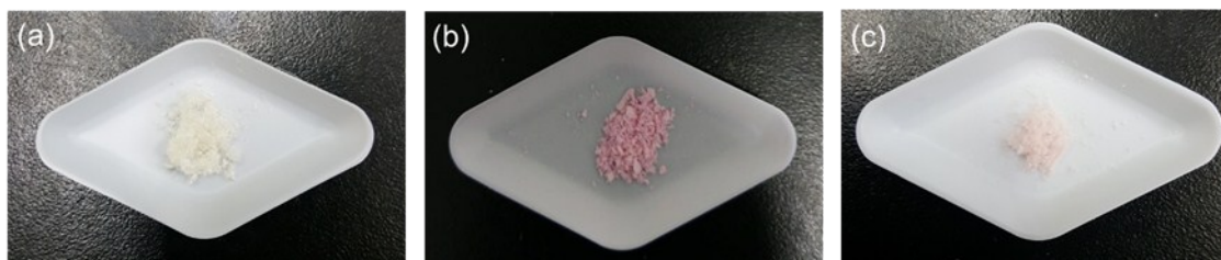
Fig. S6 Photographs of (a) as-synthesized SmBTC powder, (b) SmBTC powder after adsorption of RB, and SmBTC powder following three adsorption-desorption cycles.
