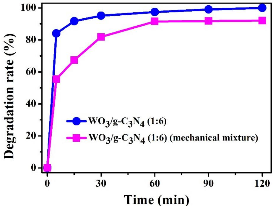
**Fig. S5** Degradation rate of CIP with  $\text{WO}_3/\text{g-C}_3\text{N}_4$  (1:6) and the mechanical mixture containing  $\text{WO}_3$  and  $\text{g-C}_3\text{N}_4$  with molar ratio 1:6 in PEF-like system, respectively.
