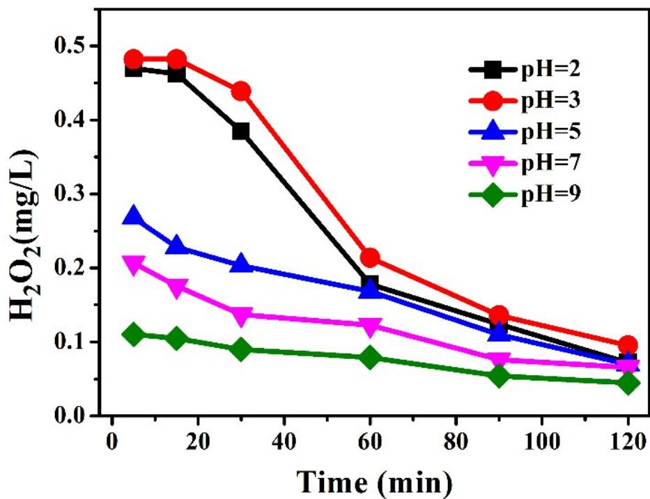
**Fig. S6** The concentration of electro-generated  $\text{H}_2\text{O}_2$  at different pH in PEF-like system with  $\text{WO}_3/\text{g-C}_3\text{N}_4$  (1:6).
