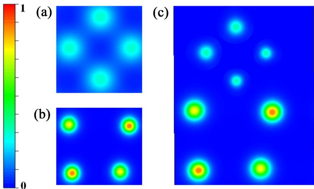
**Fig. S8** Electron density maps of  $\text{WO}_3$  (a),  $\text{g-C}_3\text{N}_4$  (b) and  $\text{WO}_3/\text{g-C}_3\text{N}_4$  model. Blue and red represented the most electro-poor and electro-rich regions, respectively.
