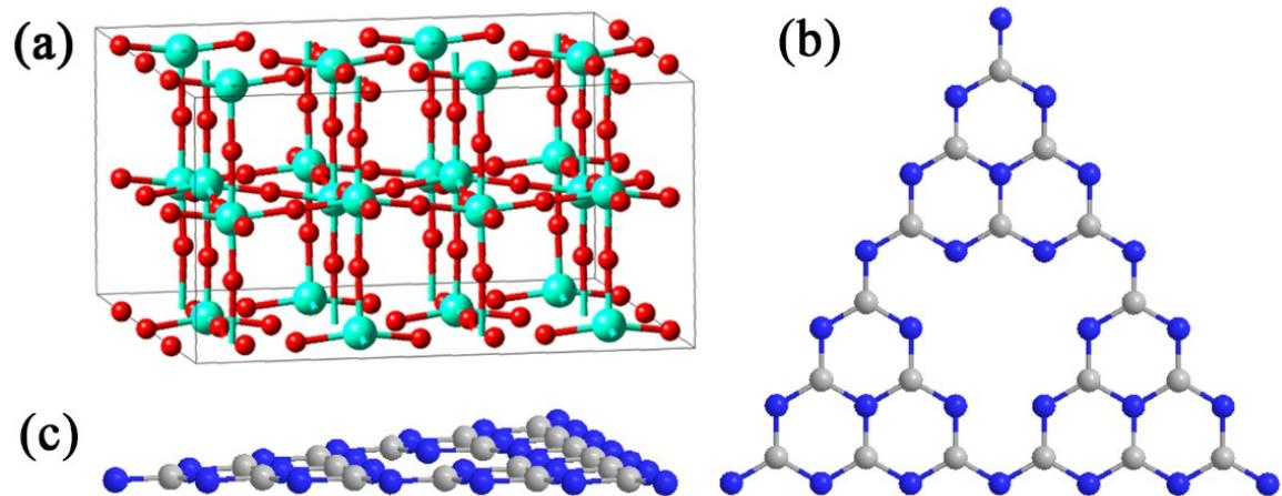
**Fig. S7** Crystal structures of monoclinic  $\text{WO}_3$  (a) and  $\text{g-C}_3\text{N}_4$  (b, c).
