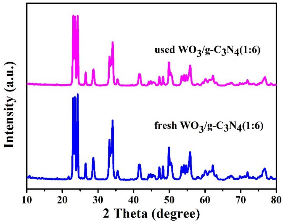
**Fig. S10** XRD patterns of fresh and used  $\text{WO}_3/\text{g-C}_3\text{N}_4$ (1:6) in PEF-like system.
