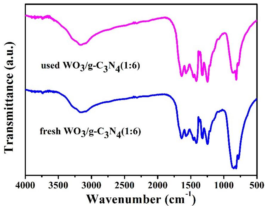
**Fig. S11** FT-IR spectrum of fresh and used WO<sub>3</sub>/g-C<sub>3</sub>N<sub>4</sub>(1:6) in PEF-like system.
