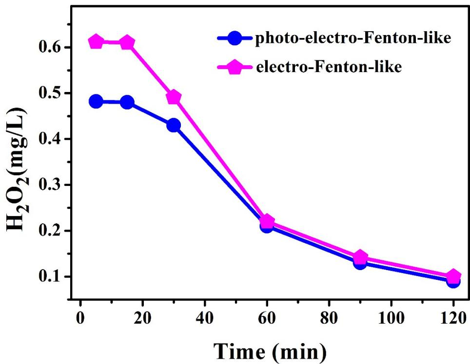
**Fig. S9** The concentration of electro-generated  $\text{H}_2\text{O}_2$  in PEF-like system and EF-like system with  $\text{WO}_3/\text{g-C}_3\text{N}_4$ (1:6).
