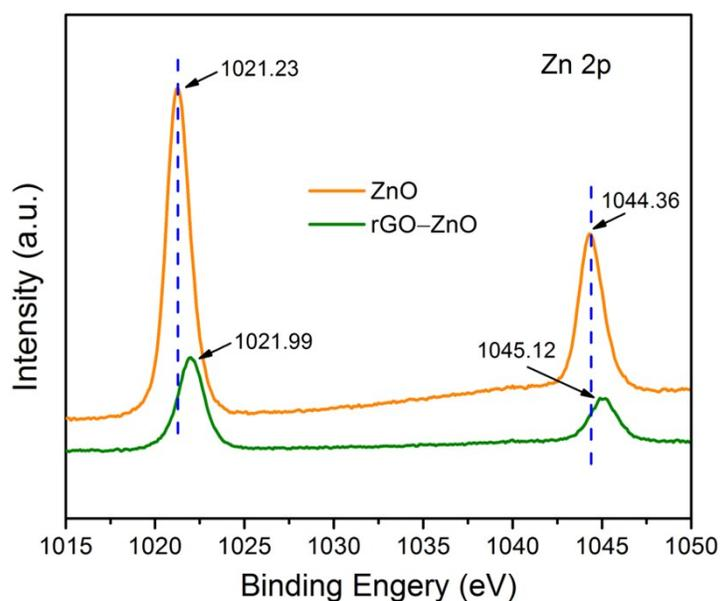
**Fig. S3** Zn 2p high-resolution XPS spectra of ZnO nanoparticles and rGO–ZnO nanocomposites. The pure ZnO nanoparticle was prepared using the sonochemical method as the rGO–ZnO nanocomposites only without GO.
