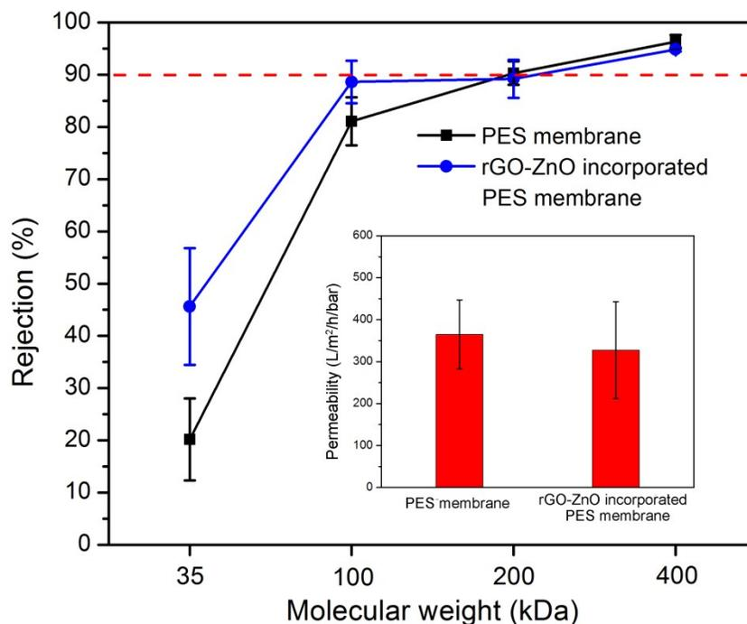
**Fig. S6** The MWCO and water permeability (insert) of pristine PES membrane and rGO-ZnO incorporated PES membrane. The values are expressed as means  $\pm$  SD,  $n = 3$ .
