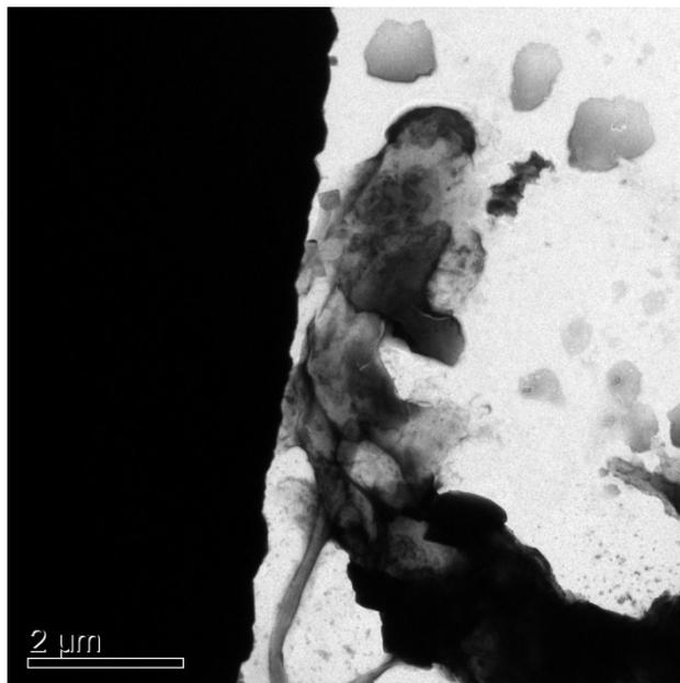
**Fig. S5** A representative TEM image of a dead bacterium after the contact killing assay on a rGO–ZnO coated PES membrane.
