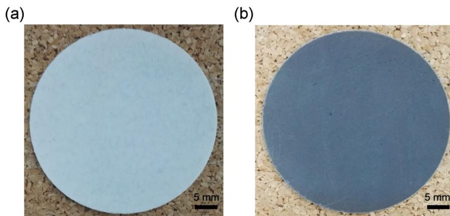
**Fig. S1** Images of a pristine PES membrane (a) and a rGO–ZnO (5% w/w) incorporated PES membrane (b) fabricated using the phase inversion method. Coupon size: 46 mm in diameter.
