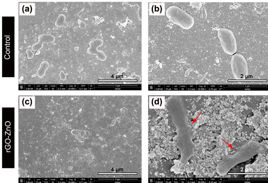
**Fig. S4** SEM images of *E. coli* following the contact killing assay on the surface of the (a–b) uncoated and (c–d) rGO–ZnO coated PES membrane.
