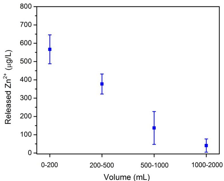
**Fig. S7** The leaching behavior of Zn<sup>2+</sup> from rGO-ZnO incorporated PES membrane (13.84 cm<sup>2</sup>) during synthetic wastewater filtration. The values are expressed as means  $\pm$  SD,  $n = 2$ .
