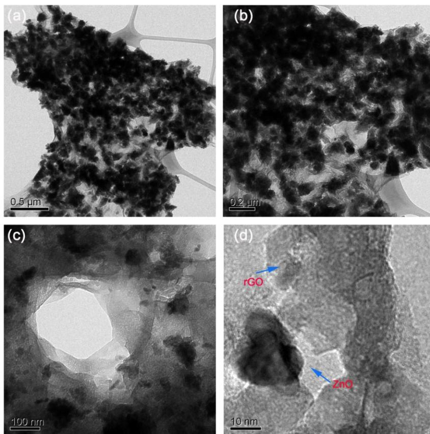
**Fig. S2** TEM images of rGO-ZnO nanocomposites at different magnifications (0.5 μm, 0.2 μm, 100 nm, and 10 nm).
