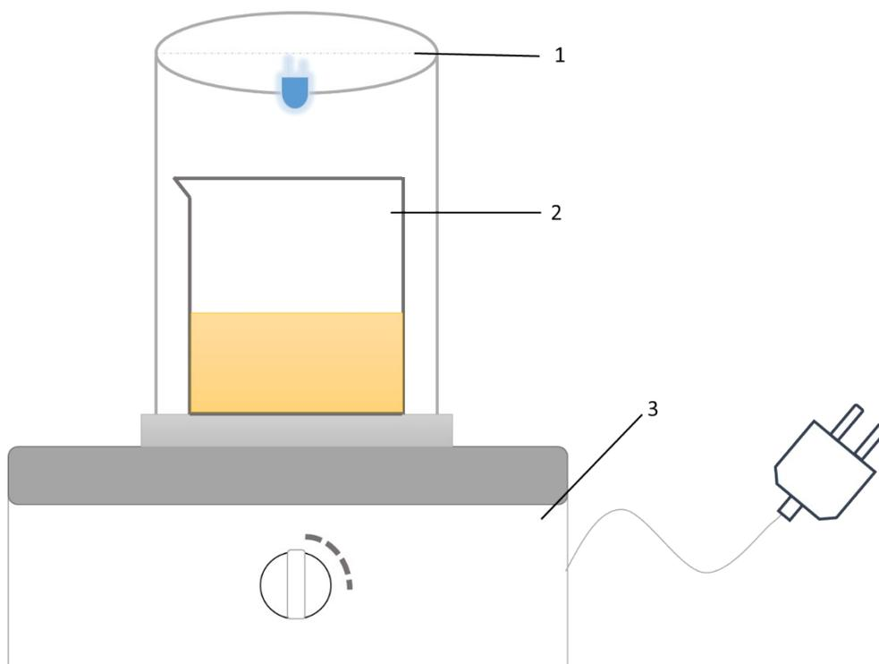
Fig. S2. Irradiation of the homemade photocatalytic reactor system: 1 = blue LED lamps, 2 = quartz breaker reaction vessel, 3 = magnetic stirrer
