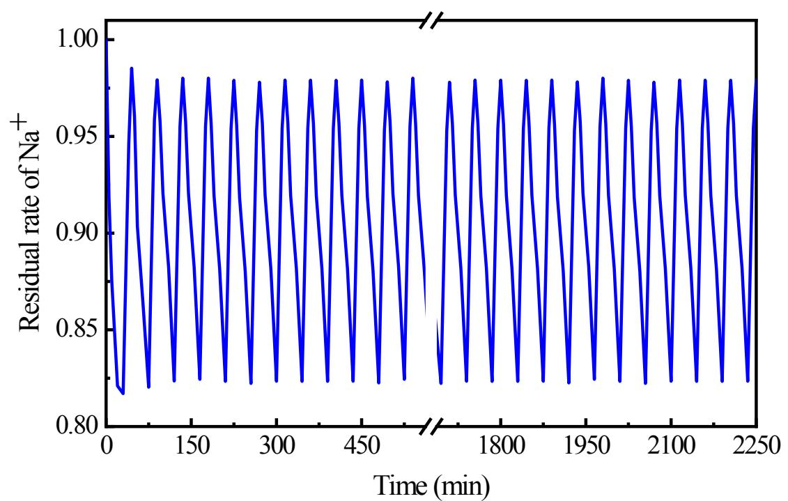
**Figure S5.** Regeneration performance of the N-GQDs@HNT electrode in batch mode using 500 mg L<sup>-1</sup> NaCl solution at 1.2 V with a flow rate of 20 mL min<sup>-1</sup>.
