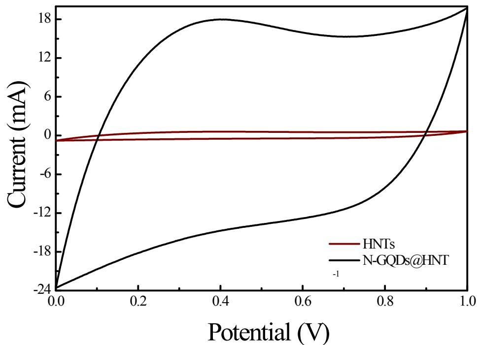
**Figure S2.** The comparison of cyclic voltammetric curves of as-received HNT and N-GQD@HNTs at a scan rate of 100 mV S<sup>-1</sup>.
