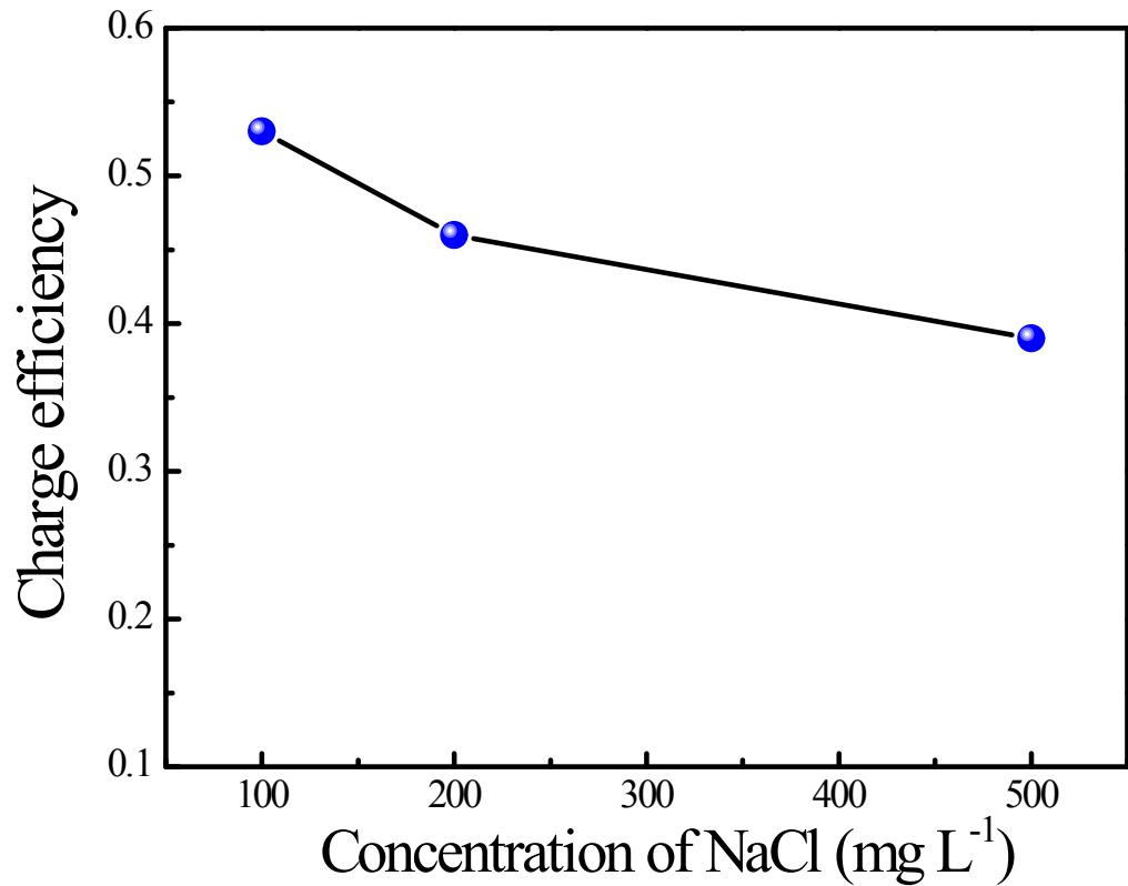
**Figure S4.** Charge efficiency of N-GQDs@HNT electrodes as a function of NaCl concentration.
