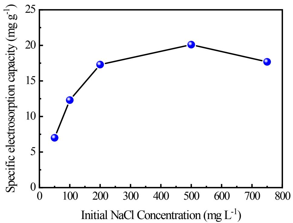
**Figure S3.** Specific electrosorption capacity (SEC) of N-GQDs@HNT at various initial NaCl concentrations.
