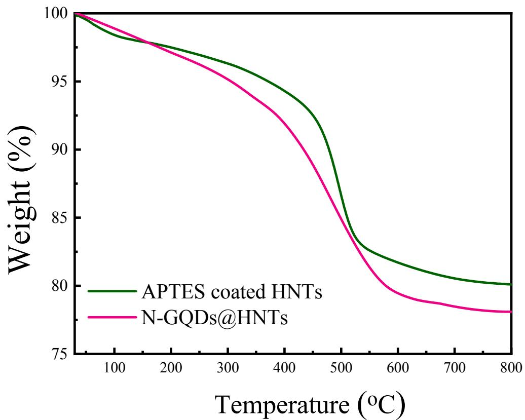
**Figure S1.** The thermogravimetric analysis (TGA) of APTES-coated HNTs and N-GQDs@HNT.
