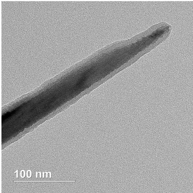
**Fig. S3.** Transmission electron microscopy image showing the single CuONW coated with polydopamine.
