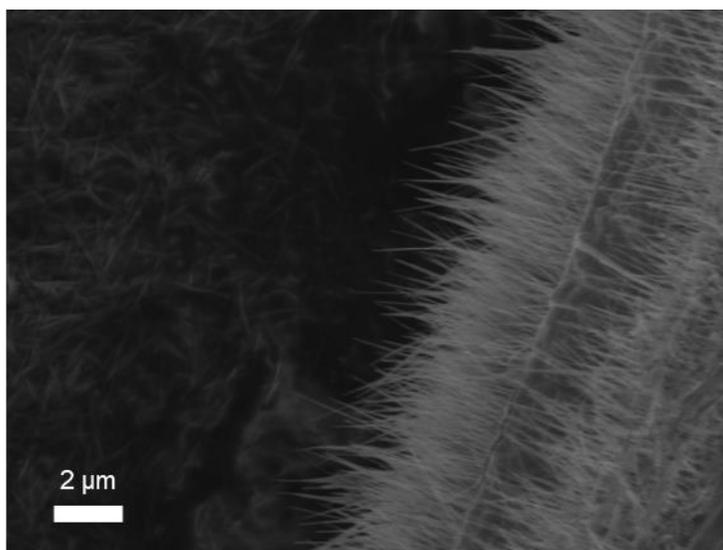
**Fig. S2.** Scanning electron microscopy image showing the bare CuONWs on the electrode surface.
