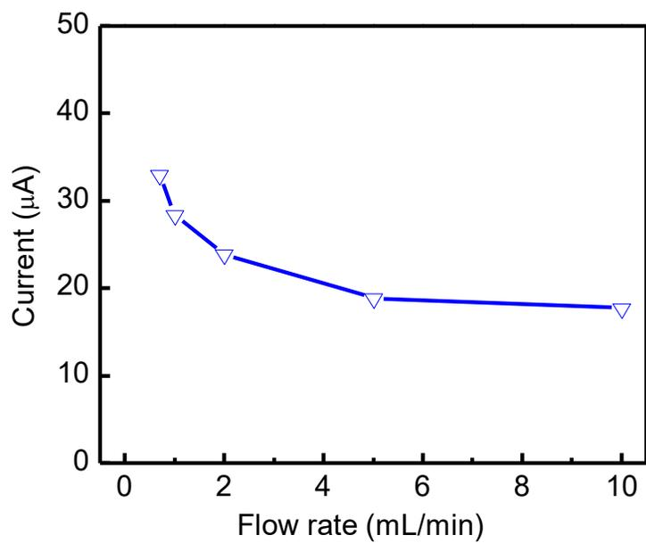
**Fig. S13.** Operating current of the LEEFT device at 1 V.
