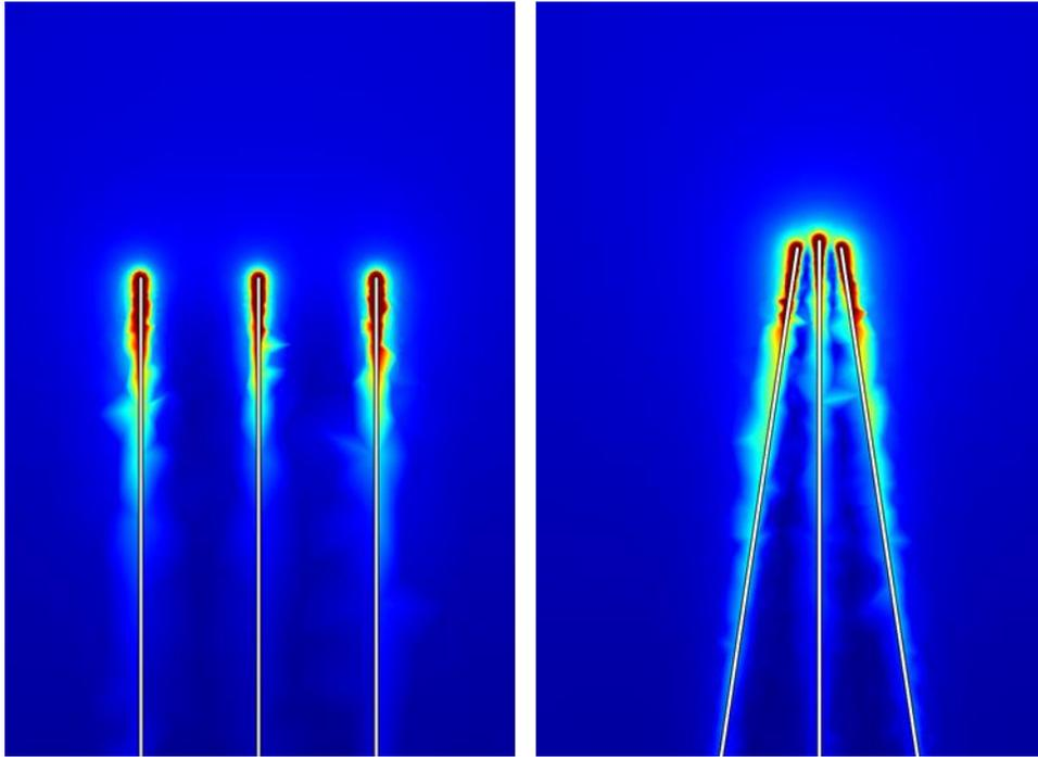
**Fig. S5.** Electric field simulation near the tip of the nanowire to study the influence of merging nanowires.
