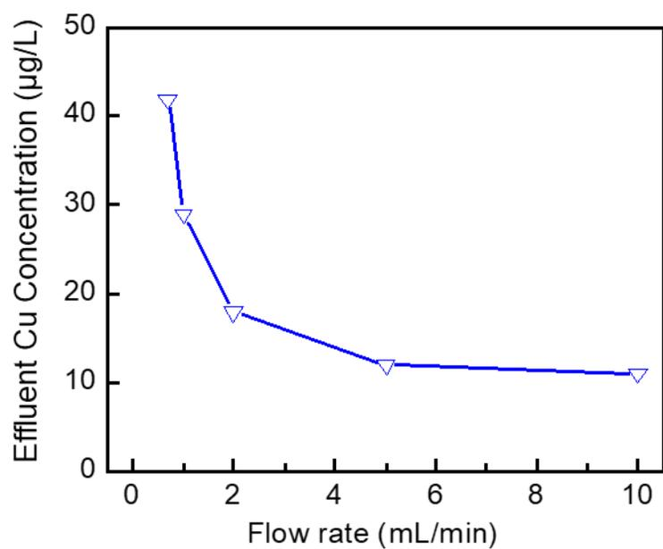
**Fig. S12.** Effluent Cu concentration of the LEEFT device with inversed current operation.
