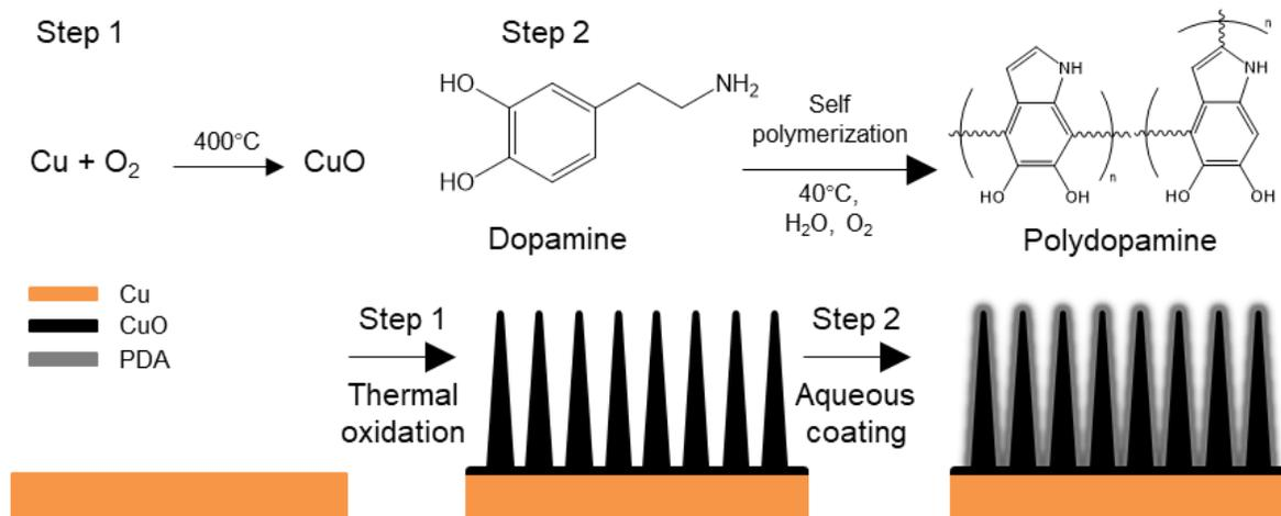
**Fig. S1.** Schematics showing the electrode fabrication processes.
