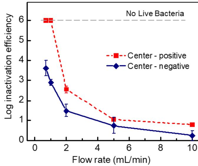
**Fig. S11.** Inactivation efficiencies of *E. coli* using an inversed electrode connection (center negative and outer positive electrodes). The applied voltage is 1 V.
