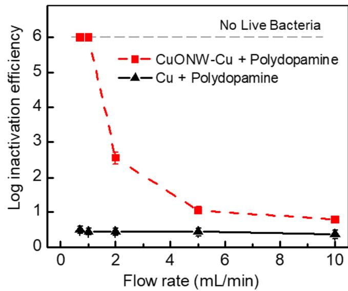
**Fig. S10.** Inactivation efficiency of *E. coli* using a polydopamine-coated copper wire as the center electrode under 1 V applied voltage.
