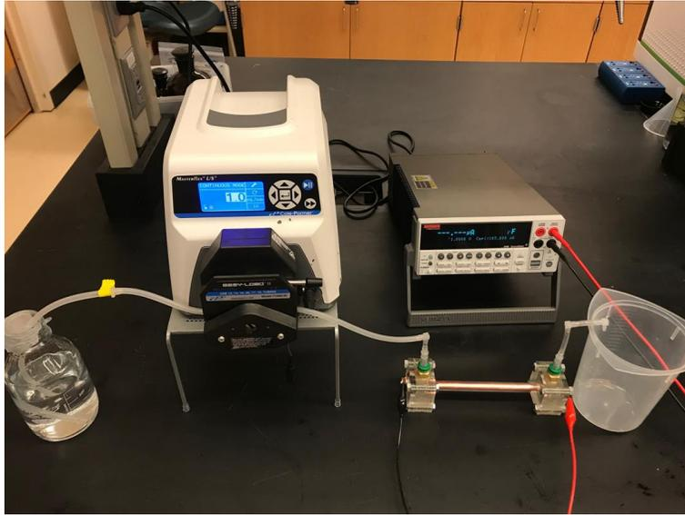
**Fig. S6.** Experimental setup of the LEEFT water disinfection.
