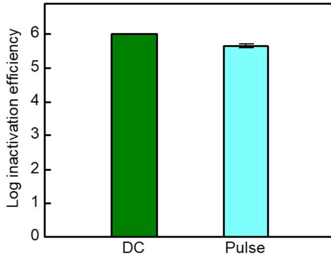
**Fig. S9.** Inactivation efficiencies of *E. coli* with direct current (DC) and pulse electric field. The peak voltage is 1V and the frequency is  $10^5$  Hz. The flow rate of the pulse treatment is 0.5 mL/min to remain the same treatment time (10 min).
