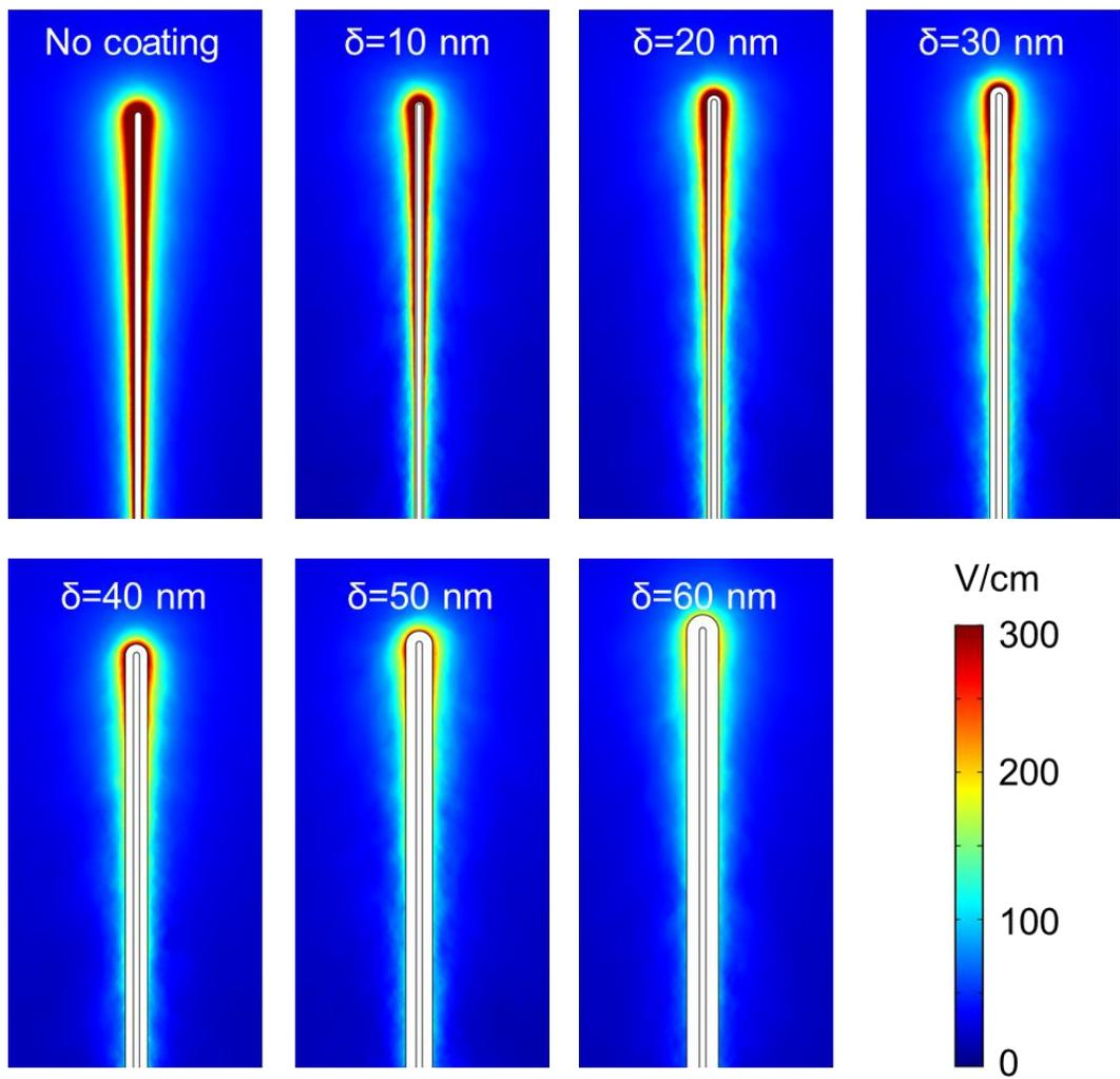
**Fig. S4.** Electric field simulation near the tip of the nanowire to study the influence of nanowire diameter. The bare nanowire has a diameter of 30 nm. The symbol  $\delta$  indicates the thicknesses of different polydopamine coating layers.
