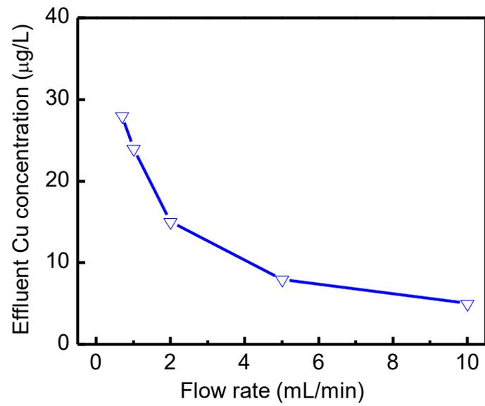
**Fig. S8.** Effluent Cu concentration of the LEEFT device operating at 1 V.
