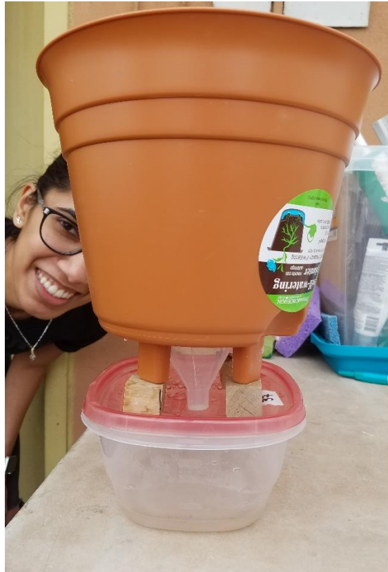
Figure S9. Leachate Collection Setup. The water flows from the pot through the funnel into the collection reservoir. The pot is elevated on wooden blocks to provide enough room for the funnel.
