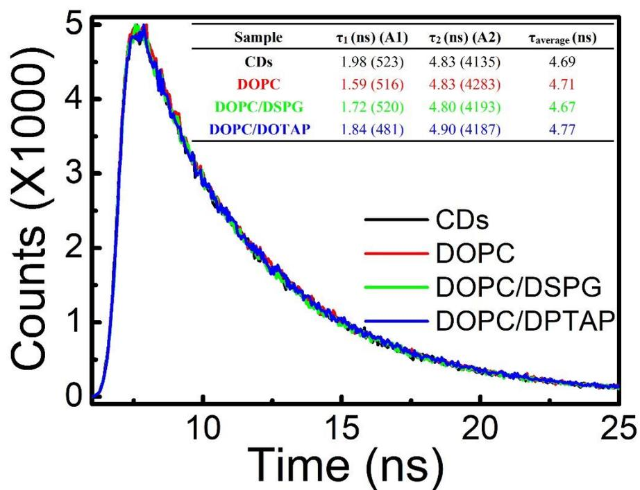
Figure S14. FL decay curves of CDs and their mixture with three kinds of liposome.  $I(t) = A_1 \exp(-t/\tau_1) + A_2 \exp(-t/\tau_2)$ ,  $\tau_{\text{average}} = (A_1 \tau_1^2 + A_2 \tau_2^2) / (A_1 \tau_1 + A_2 \tau_2)$ .
